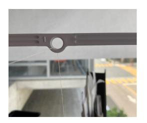
2. Pass the thread through the corresponding thread guide
