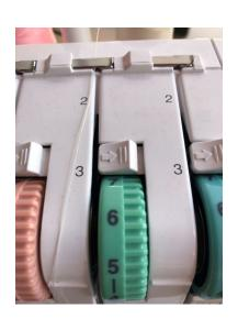
4. Guide the thread down the channel and through the hooks following the green line
