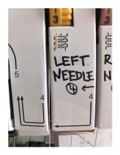
6. Bring the thread down through the guide above the needle and through the left needle from front to back
