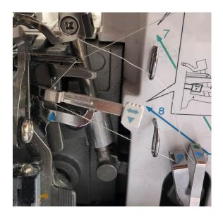
6. Position the thread under the hook (left end) of the threading lever
