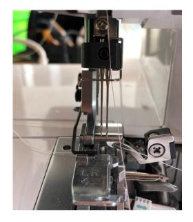
6. Bring the thread down through the guide above the needle and through the right needle from front to back
