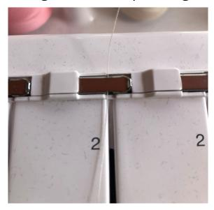
3. Slide and hold thread tension release button to the right, then pass the thread through the tension disc, release the button
