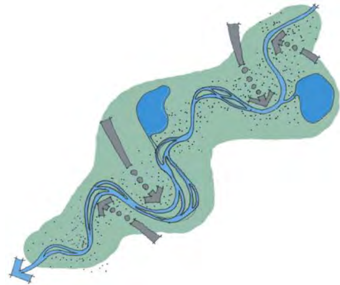
Re-contour the channel to increase the river's length and meander, expand ground water recharge area, separate ponds from the River, and filter urban run-off before it reaches the river
