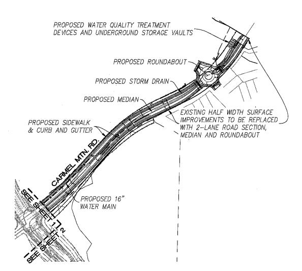
T-5.2: CARMEL MOUNTAIN ROAD, 2 LANE MODIFIED COLLECTOR FROM SR-56 TO CAMINO DEL SUR. GRADE AND CONSTRUCT ROAD IMPROVEMENTS INCLUDING STORM DRAIN, WATER QUALITY AND HYDROMODIFICATION MEASURES, EROSION CONTROL, CURB AND GUTTER, SIDEWALKS, PAVEMENT, LANDSCAPE & IRRIGATION, TRAFFIC CONTROLS, SIGNING, STRIPING, AND ROUNDABOUT.
