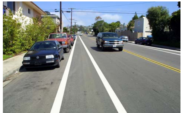
Above: Phase One bike lane markings. These lanes are added to La Jolla Hermosa as an example of the visual effects of narrowed travel lanes. As a general rule, most motorists respond to 10.0 foot lanes by driving about 7 mph lower speeds.
