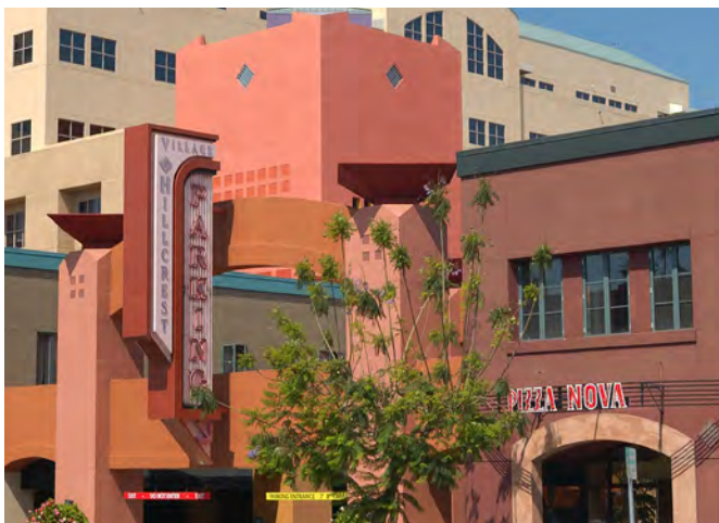
Entrances to parking garages should be integrated into building design and isolated from primary pedestrian entrances, if possible.
