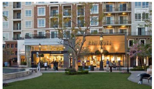
Figure 4.1e - Maintain consistent massing and perceived building height at the street level, and break up long unbroken façades with offsets and articulations.
