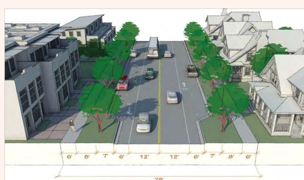
PLACEHOLDER GRAPHIC: Illustrative cross-section with right-of-way dimensions
