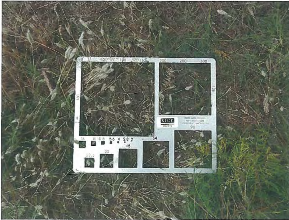
Figure 5: Basin 900 Reach 2 - Gravelometer on Channel Bed
