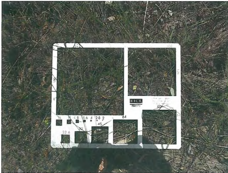
Figure 11: Basin 1000 Reach 4 Gravelometer on Channel Bed
