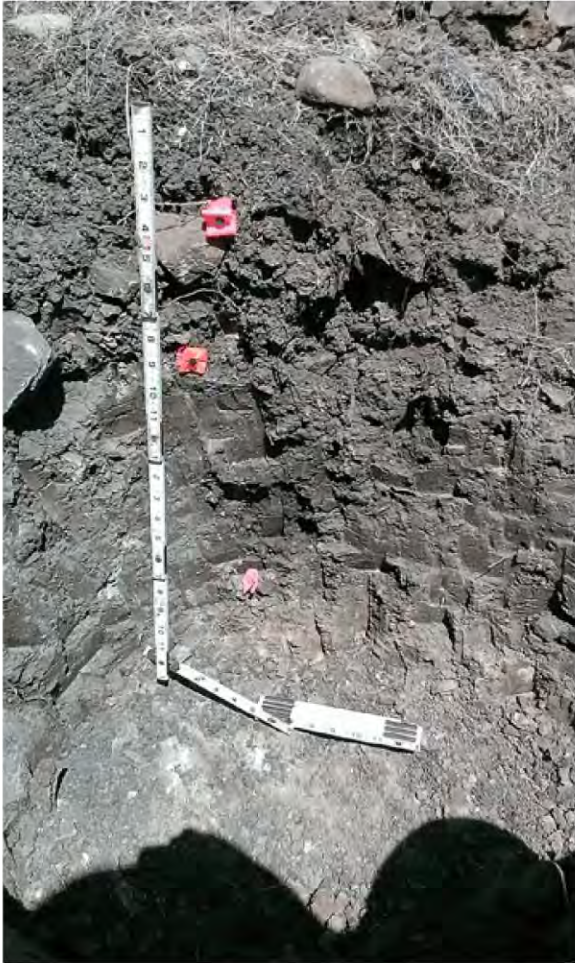
Figure 3 Gravel to cobble size rock fragments exposed in Test Pit TP-3. The transition for dessicated, granular to medium subangular, and underlying "massive" structure is indicated at approximately 9 inches on the scale. Please note that this transition is deeper on the opposite side of the pit, as indicated on the log for TP-3.
