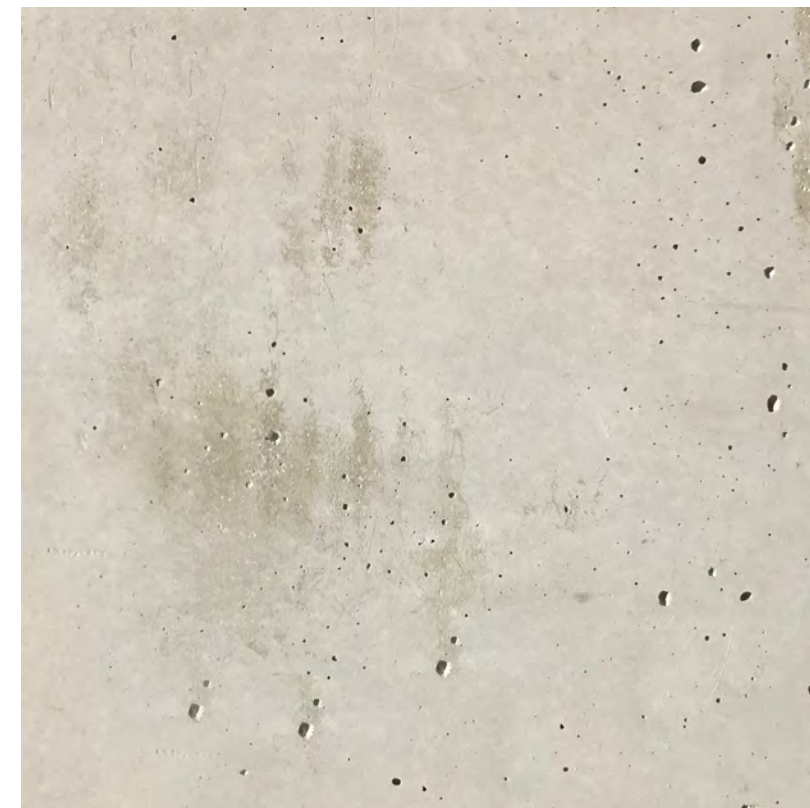
(CO) ARCHITECTURAL CONCRETE TYPE 1L - "WHITE" CONCRETE WITH WARM HUES, EXPOSED AND ARCHITECTURAL GRADE
