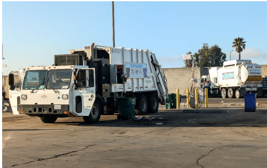
Figure 9-1 Rear Load Compressed Natural Gas Truck at Miramar Yard
