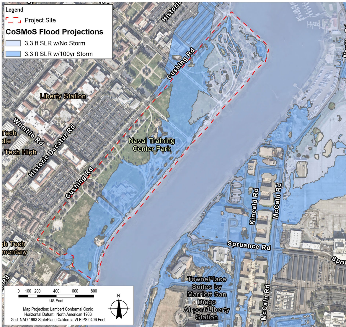
Figure 23. USGS CoSMoS flood hazards with 3.3 ft of sea-level rise with and without a 100-yr storm
