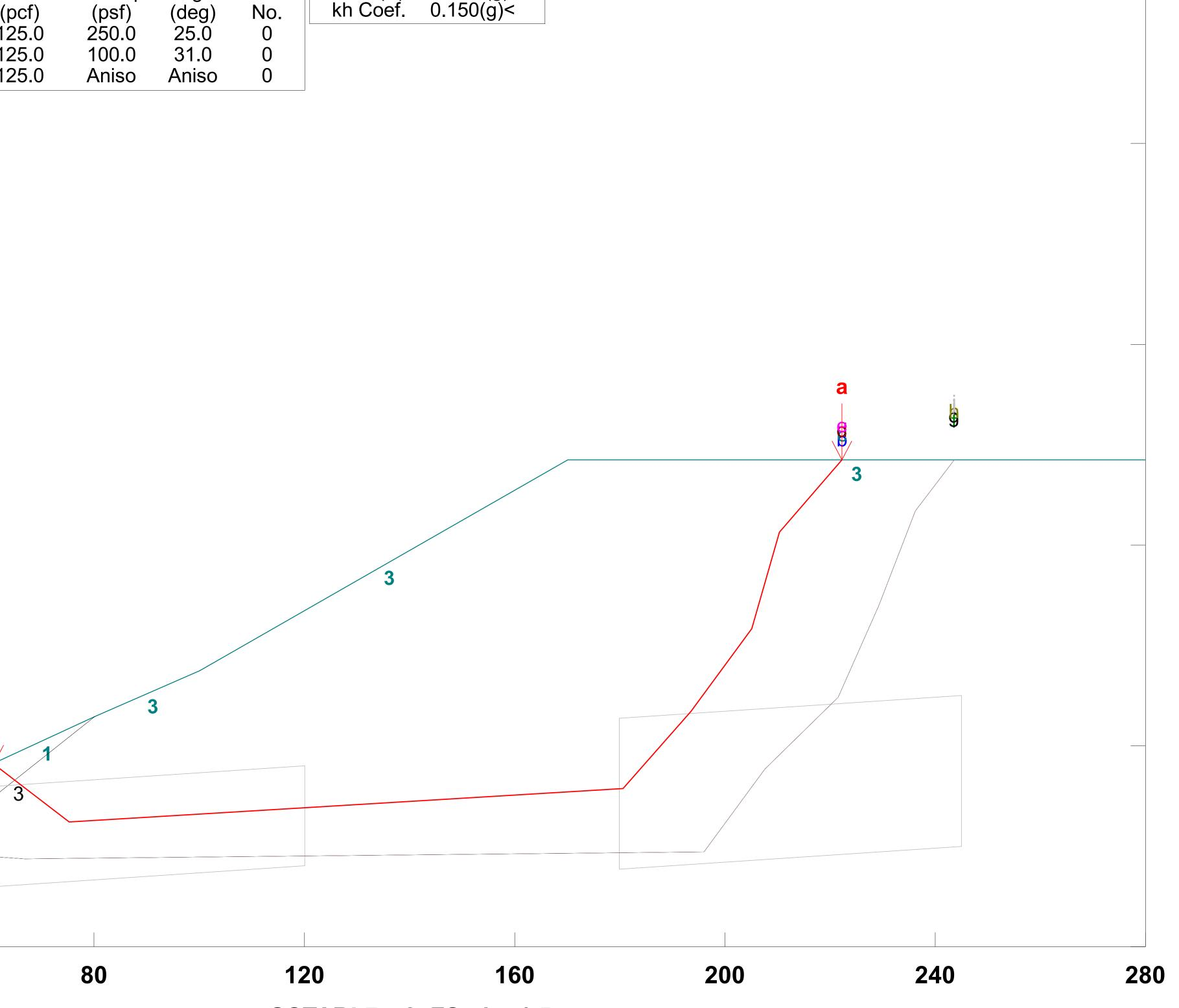
GSTABL7 v.2 FSmin=1.5 Safety Factors Are Calculated By The Simplified Janbu Method for the case of c & phi both > 0
