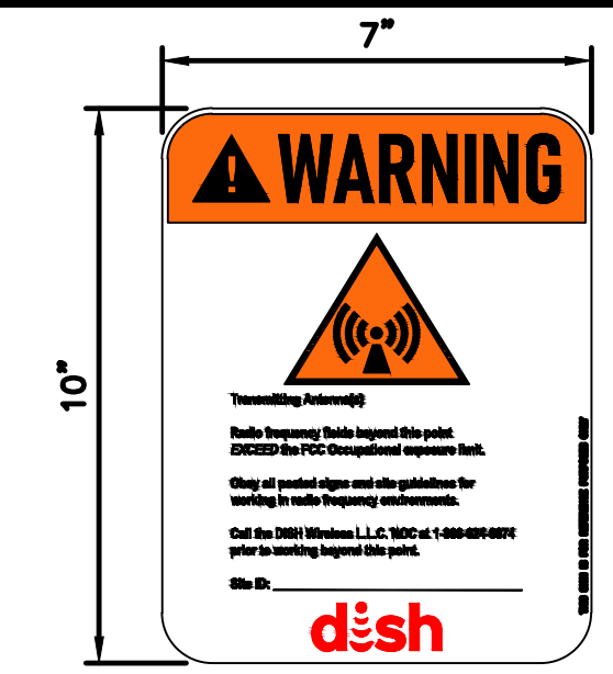
NEW SIGNAGE TO BE INSTALLED 10' ABOVE GROUND LEVEL AT THE BASE OF THE LIGHT POLES
