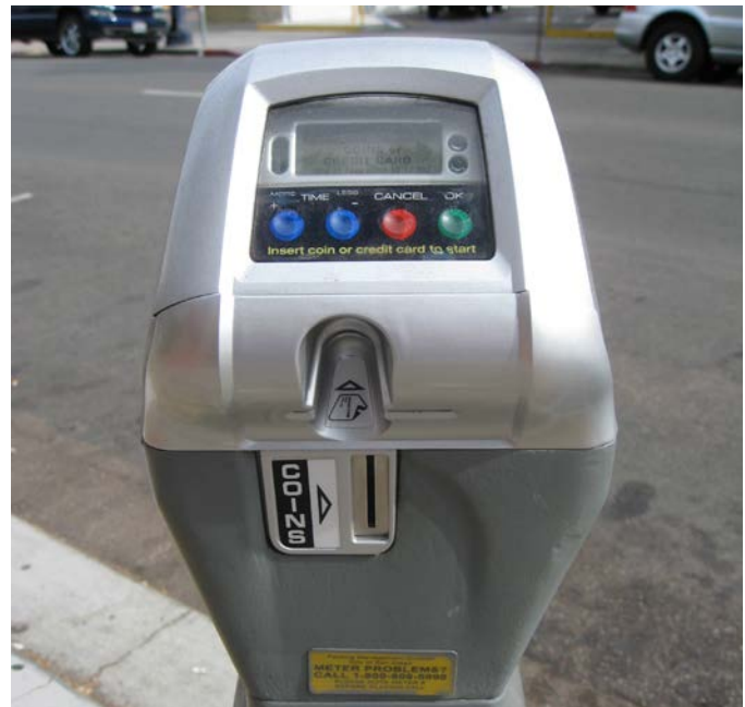
Electronic parking meters can provide adjustable time duration rates and statistical data on parking utilization.
