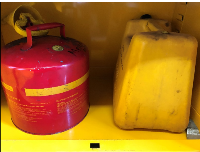
11. View of gasoline and oil stored in secondary containment within maintenance shed
