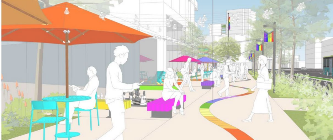
12 inches wide band of Multi-colored (min. 3 colors) paving
