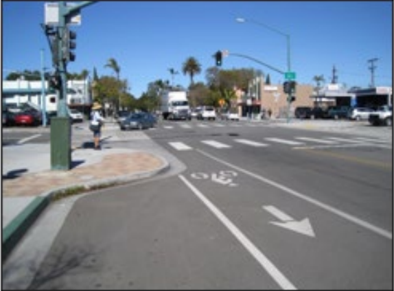
Curb Extension / Bulb-outs
