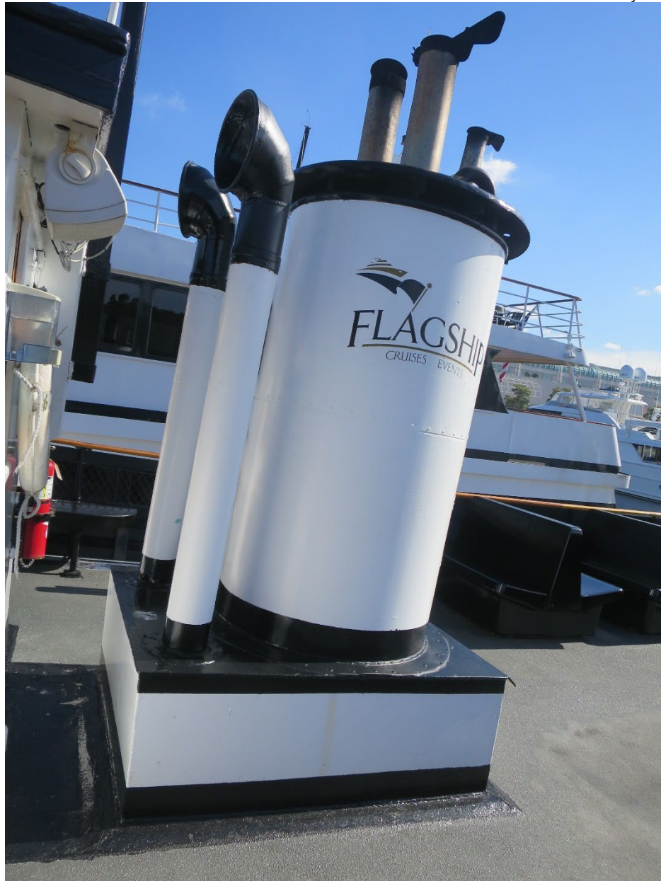
Photo 15. Silvergate , upper deck, starboard view showing smokestack enclosure and apron
