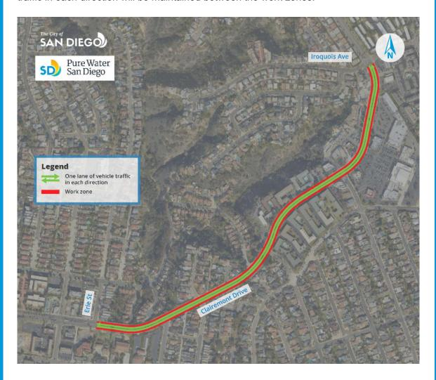
During stage 2, crews will pave the inside lanes of Clairemont Drive, and one lane of traffic in each direction will be maintained on either side of the work zone.
