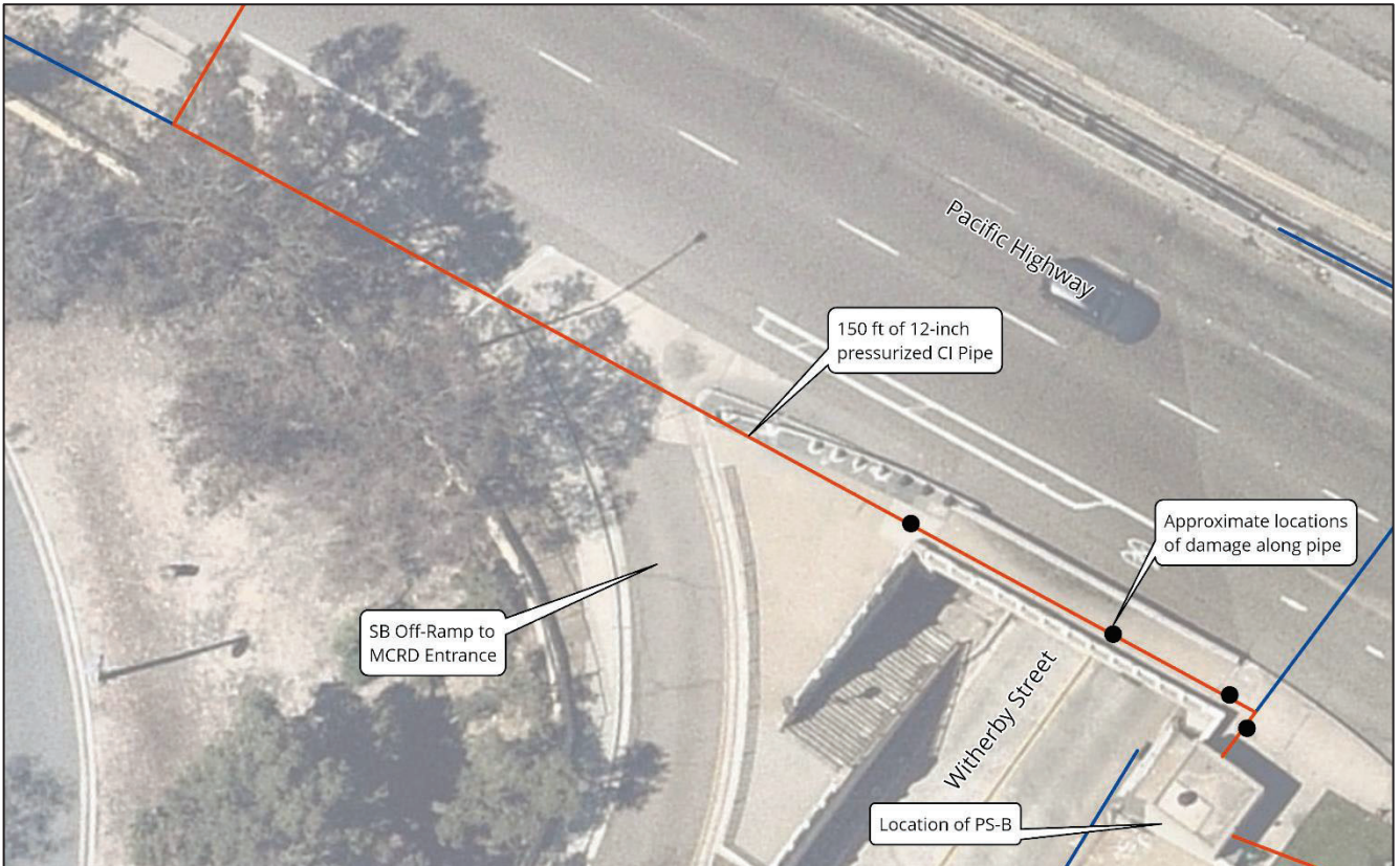
Damages Along Northern Pressurized RCP Exhibit
