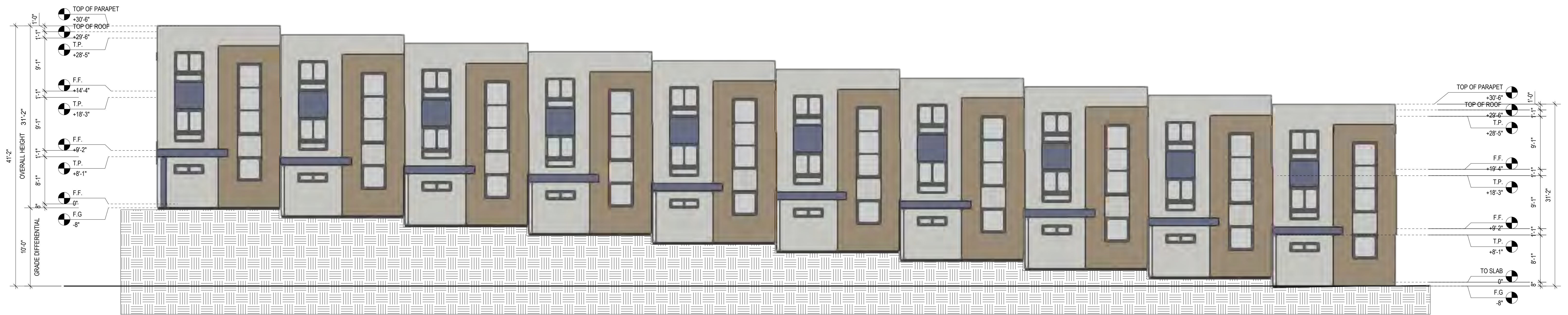
1 SOUTH OVERALL ELEVATION (FRONT UNITS) Scale: 1/8" = 1'-0"
