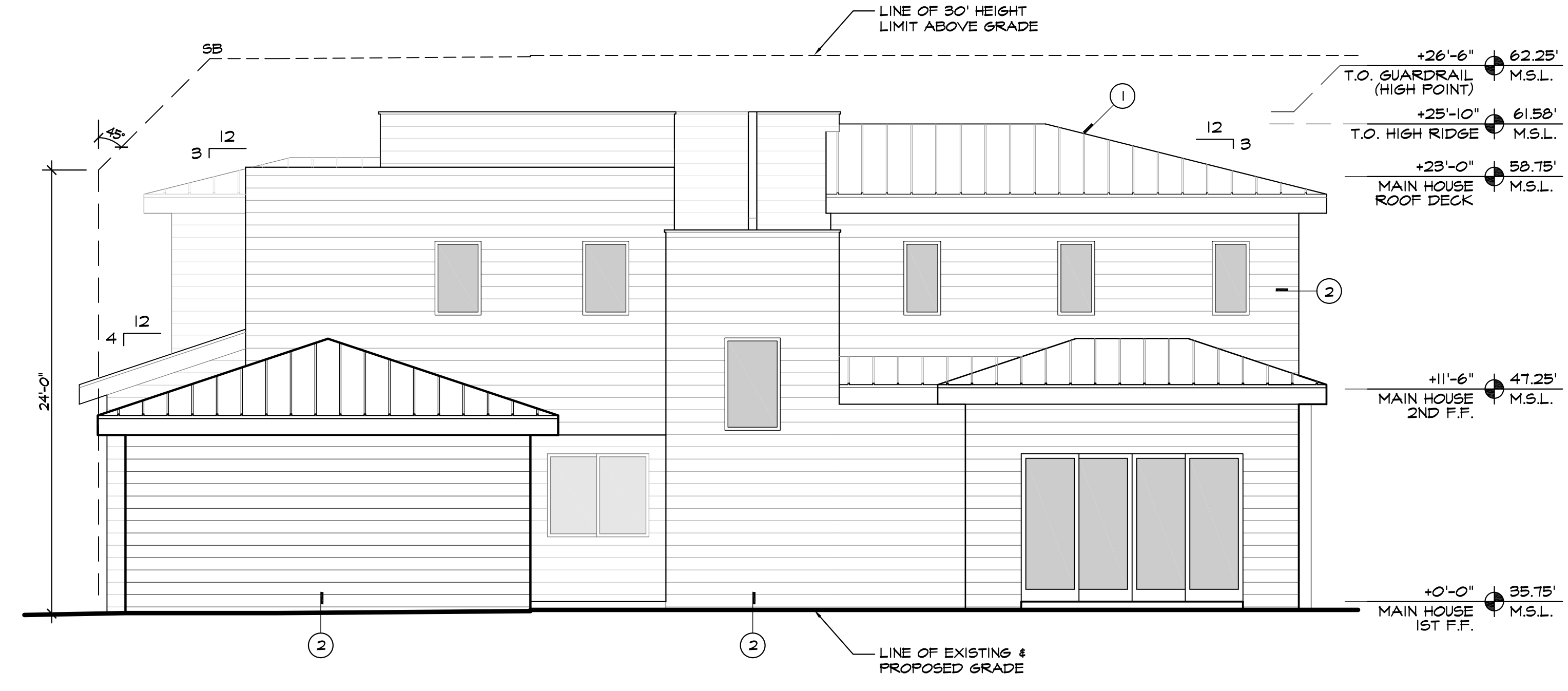
EAST ELEVATION - MAIN HOUSE SCALE: 3/16"=1'-0"
