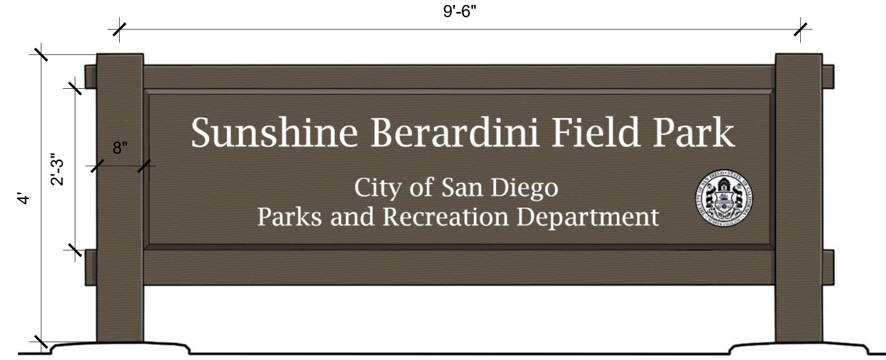
ENTRY MONUMENT SIGN, SCALE: 3/4" = 1' Precast concrete with faux wood texture
