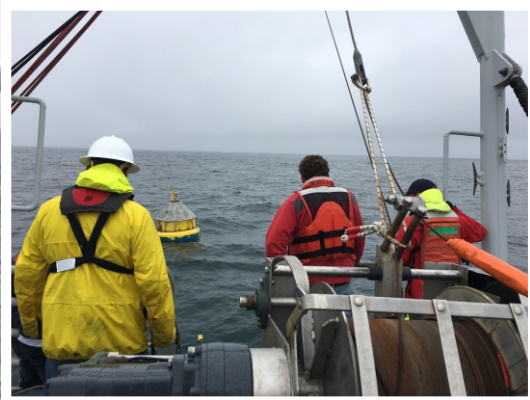
Scripps Institution of Oceanography researchers joined City Staff to assist in the deployment of our Real-Time Oceanographic Mooring System (RTOMS).
