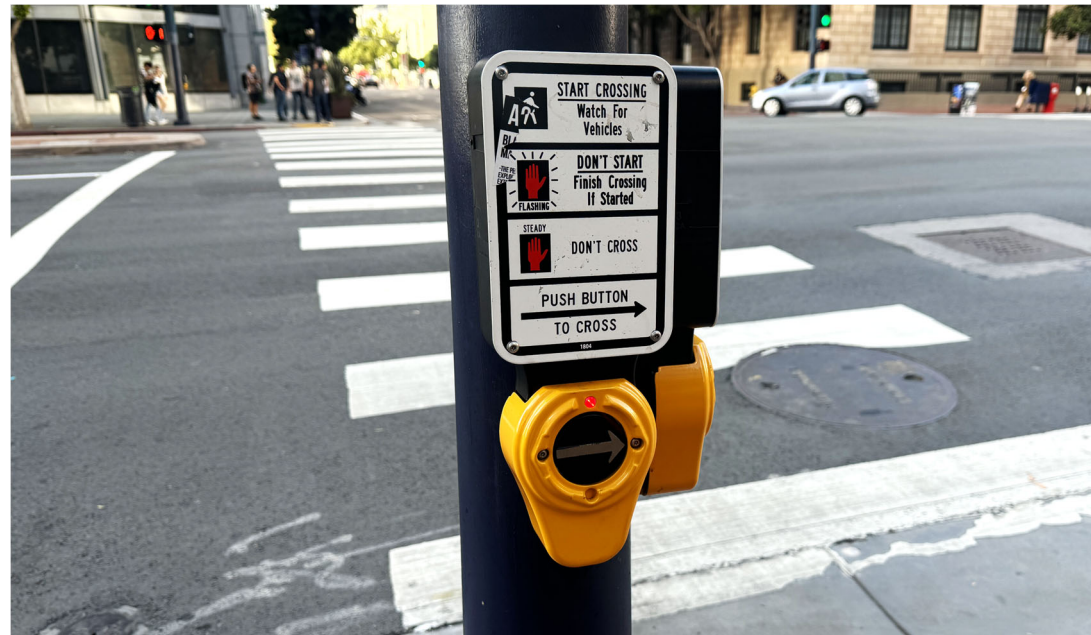
FIGURE 6-19 ACCESSIBLE PEDESTRIAN SIGNAL
