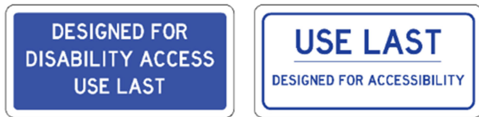
FIGURE 3-11 ELECTRIC VEHICLE ACCESSIBILITY CHARGING SIGN
