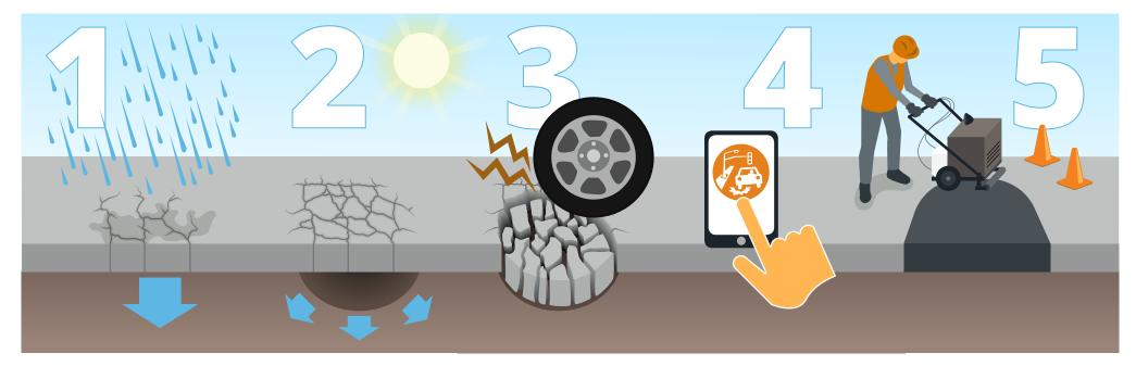
**1**. Cracks caused by traffic and aging allow rainwater to seep through and erode pavement base.
