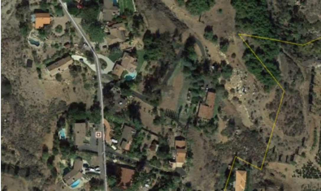
Figure 5. Example of “moderate density” development. Homes are located on larger properties and include varying levels of ignition resistance and landscape / fuel modification provision and maintenance. This type of development results in a higher wildland exposure level for all homes and does not provide the same buffers from wildfire encroaching onto the site, or starting at a structure and moving into the wildlands as a higher density project.
