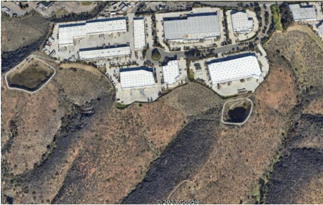
Figure 5. Example higher density development. Homes are ignition resistant and excludes readily ignitable vegetative fuels throughout and provides a perimeter fuel modification zone. This type of new development requires fewer fire resources to defend and can minimize the likelihood of on-site fires spreading off-site.
