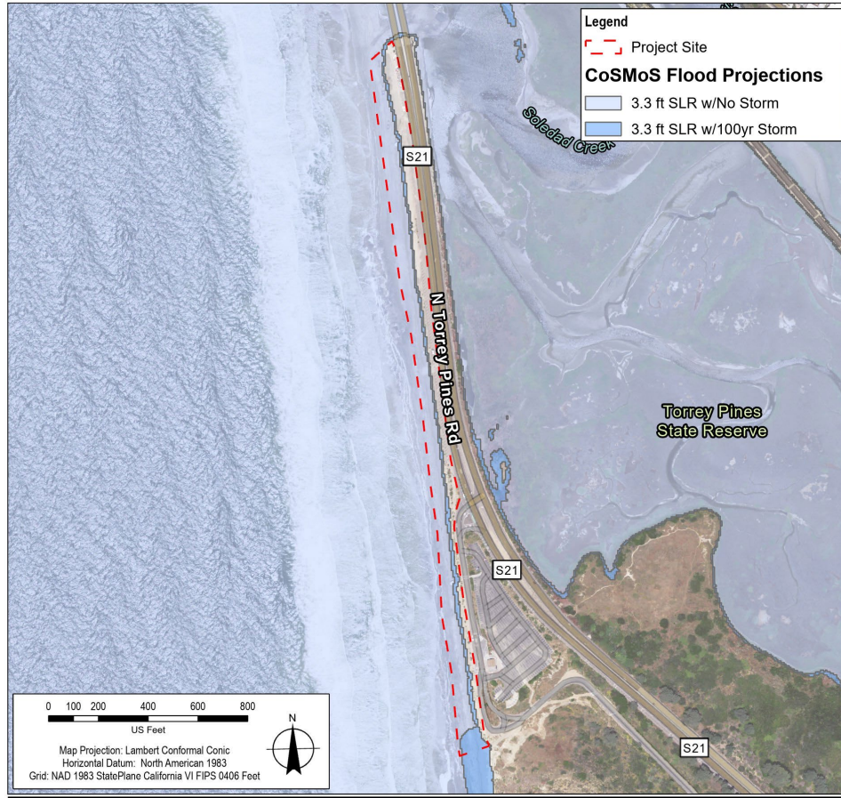
Figure 3. USGS CoSMoS flood hazards with 3.3 ft of sea-level rise with and without a 100-yr storm
