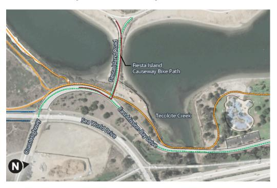
0→0 ↑ ↓ 0←0 Construct separate bike lanes and a 16-foot multi-use trail with a 2-percent maximum cross-slope using one of several configurations
