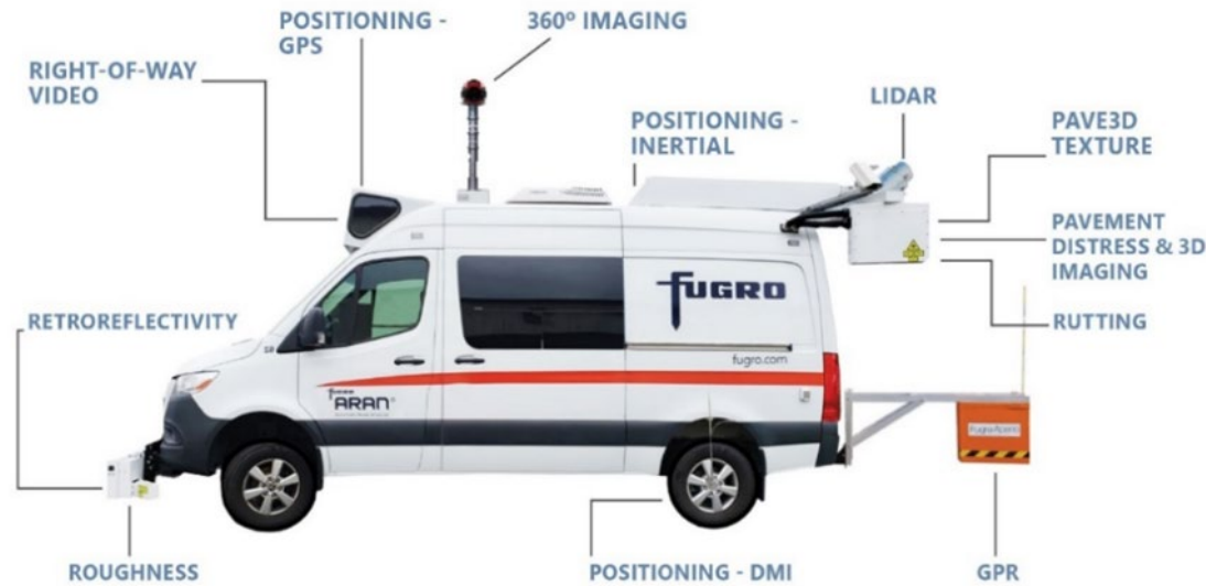
Figure 1. Fugro's ARAN Sub-Systems Overview
