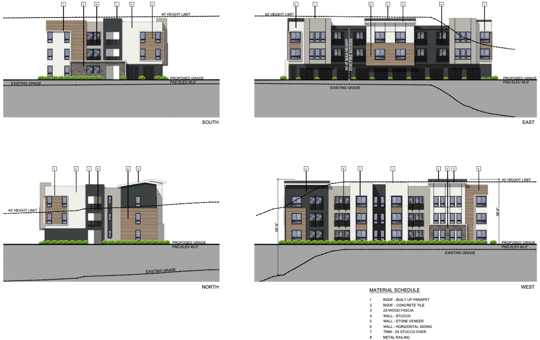
Figure 3-2a. Project Elevations – Building A Elevation
