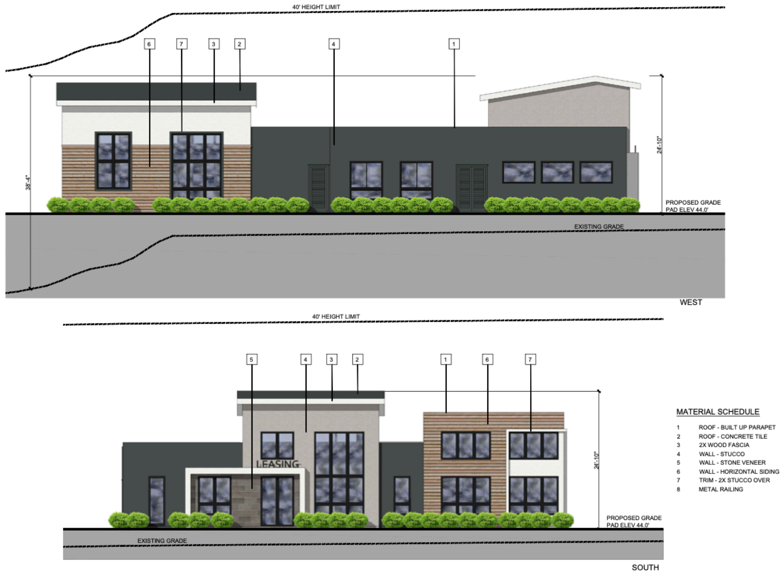
Figure 3-2g. Project Elevations – Rec/Leasing Building Elevation
