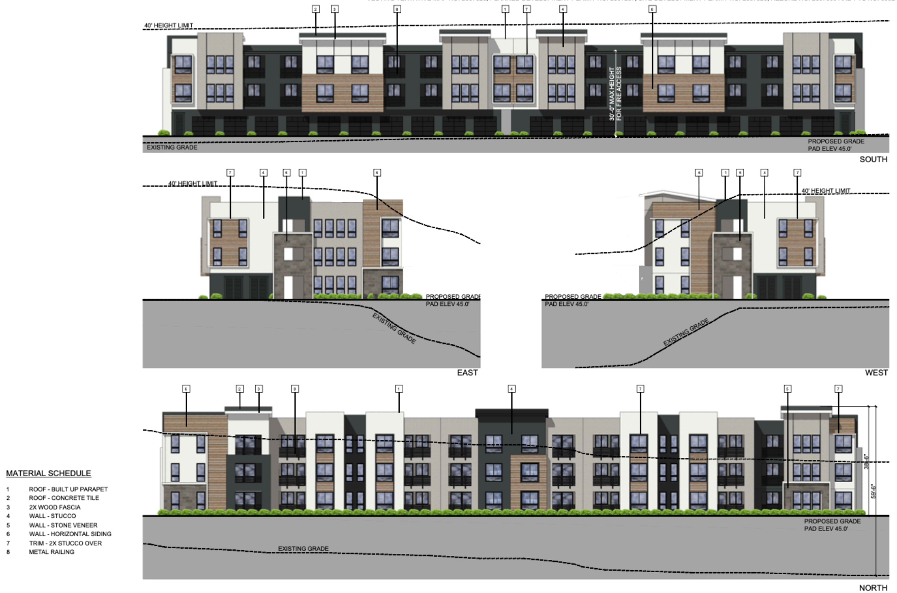
Figure 3-2c. Project Elevations – Building C Elevation Building 2
