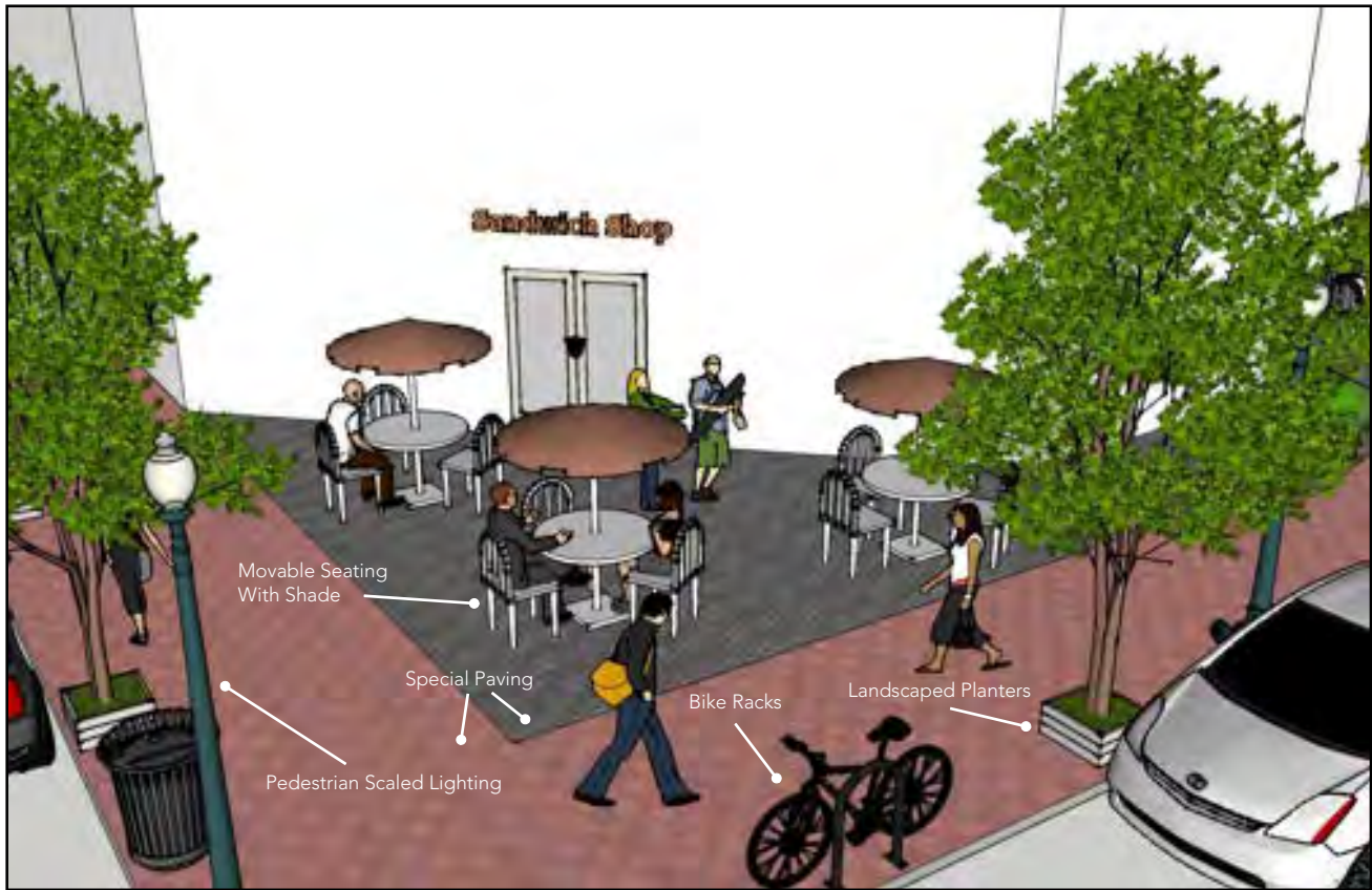
Figure 4.3 Chamfered Corners with outdoor seating
