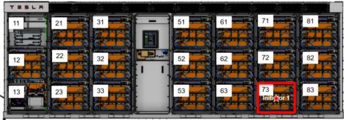
Fig 4. Initiator AC Battery module location
