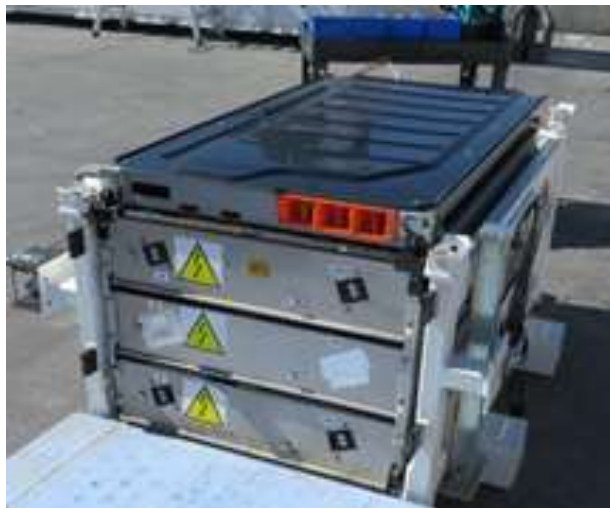
Fig 10. Initiator Qbert module, Rear view – Post test
