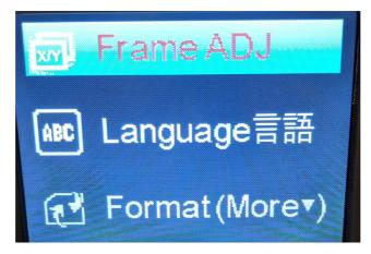
Once in the Frame Adjustment window, use the **"Enter"** button to move and select the *Y*, *X* or *W* options. Then use the up and down arrows to change the value to adjust frame, such as moving the frame left or right. Once you are happy with setting up your frame click the Menu button to exit Frame ADJ option.
