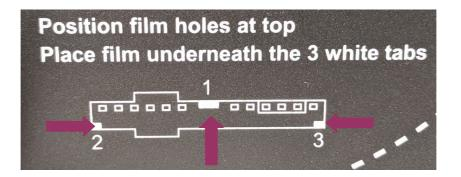
Once film is aligned underneath the 3 white tabs, you can close the latch. Then slide the film type button (see green box) to select either 8mm or Super8 film.
