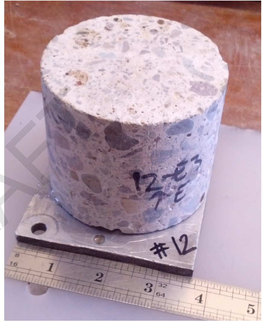
Core #12: As-received profile section mounted on Al base plate
