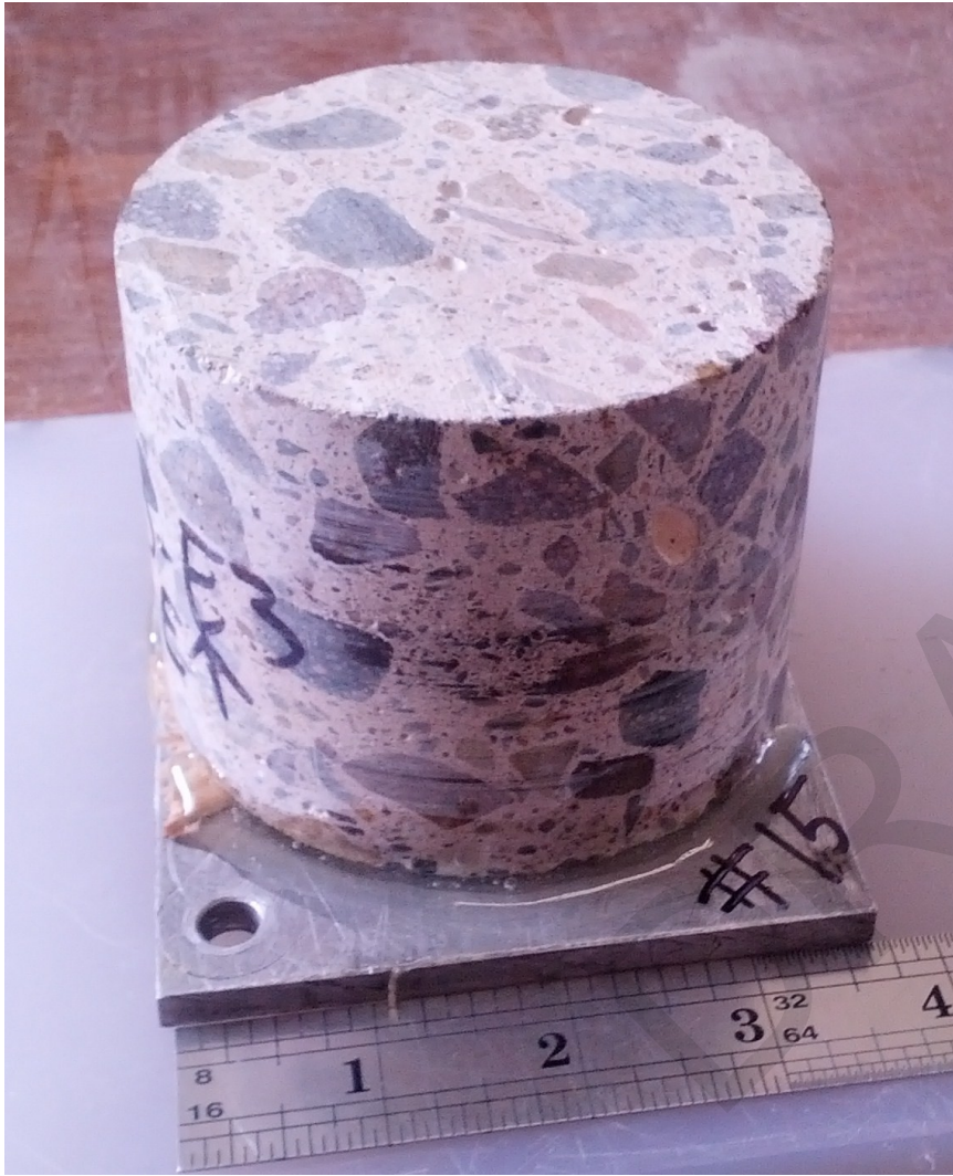
Core #15: As-received profile section mounted on Al base plate
