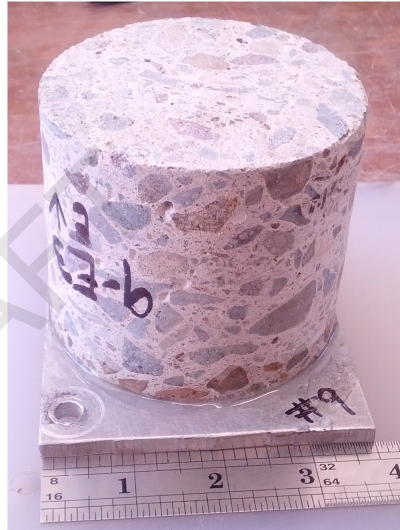
Core #9: Section for chloride analysis was cut at 2 1/2" from the exposure surface. No reinforcement was observed.
