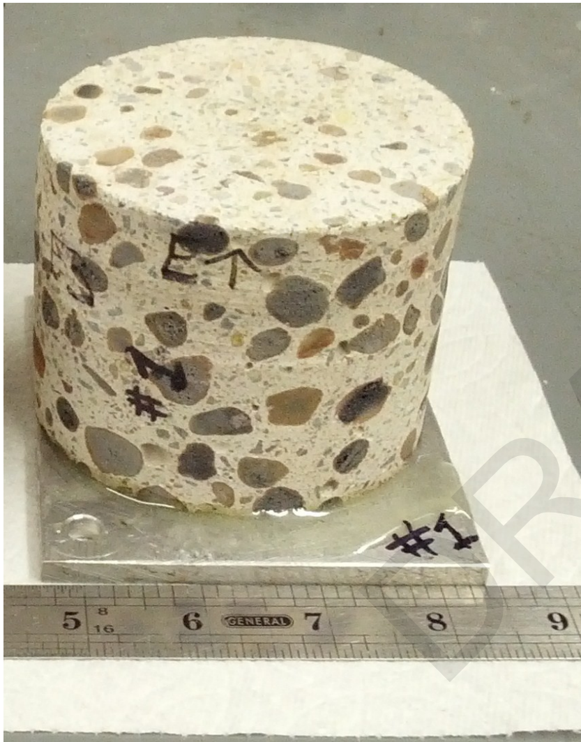
Core #1: As-received profile section mounted on Al base plate
