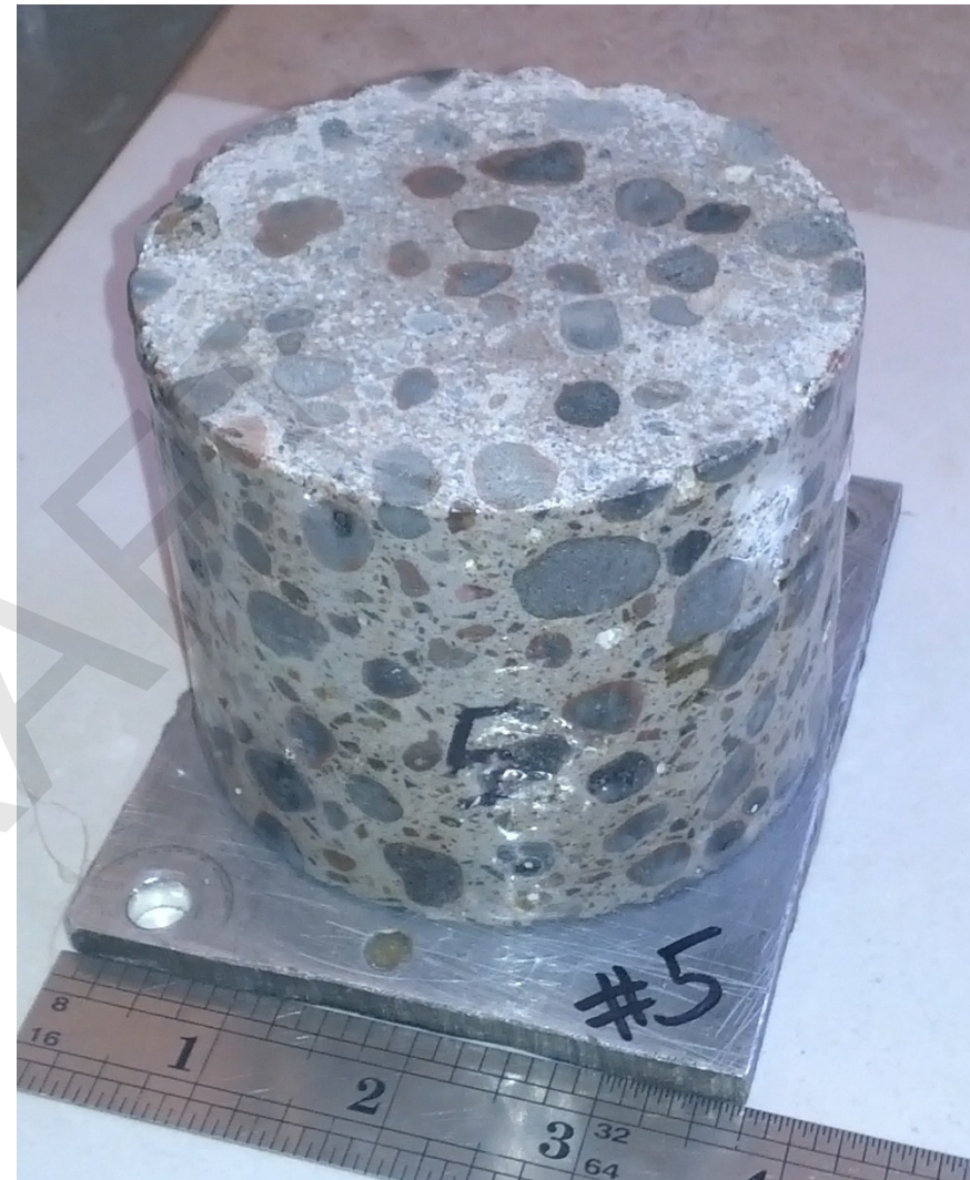
Exposure core #5: As-received profile section mounted on Al base plate
