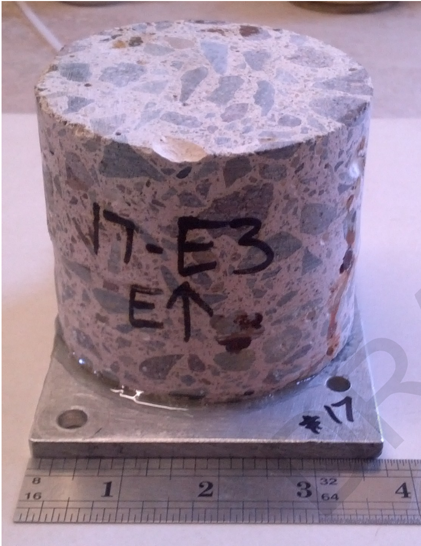
Core #17: Section for chloride analysis was cut at the observed reinforcement level. Reinforcement is located at about 1 \frac{3}{4} " below the exposure surface.
