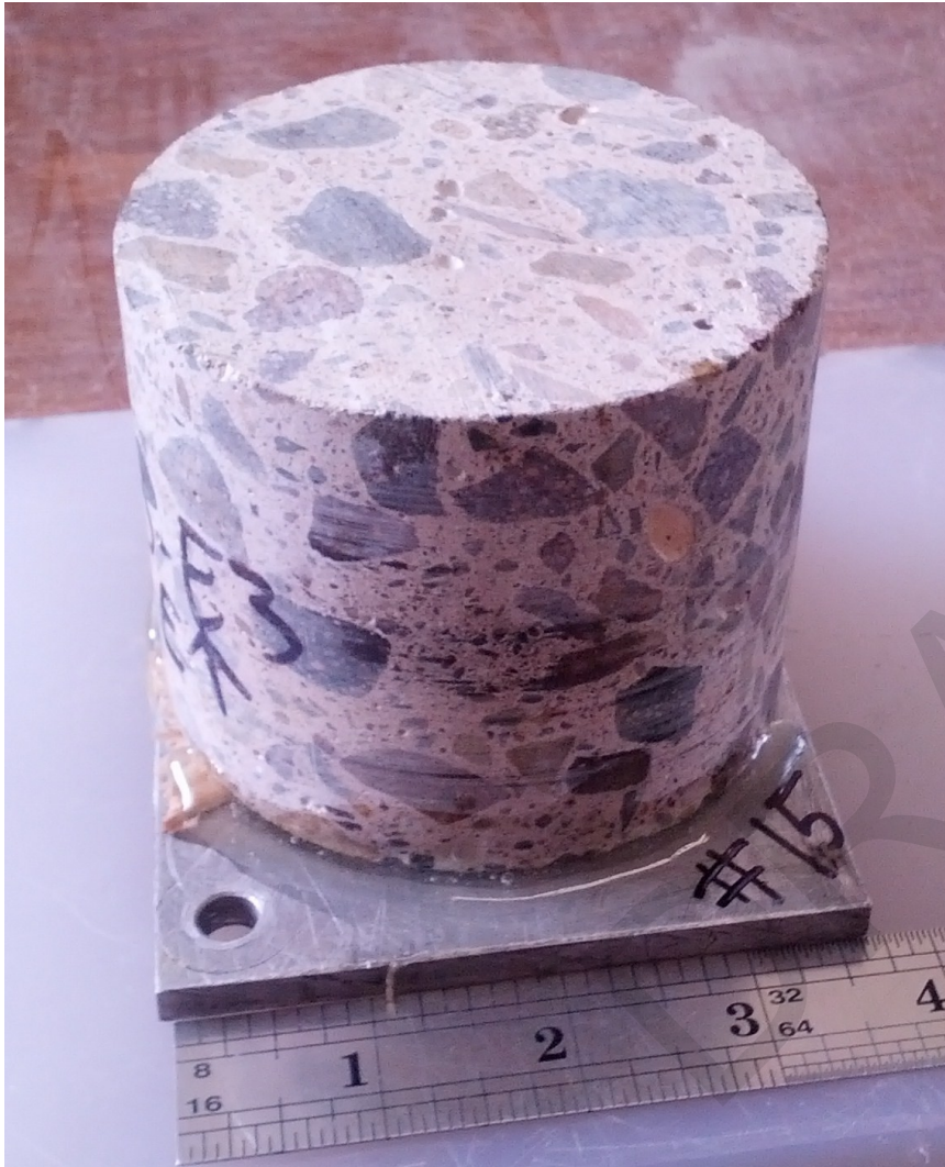
Core #15: Section for chloride analysis was cut at the observed reinforcement level. Reinforcement is located at about 2 1/4" below the exposure surface.
