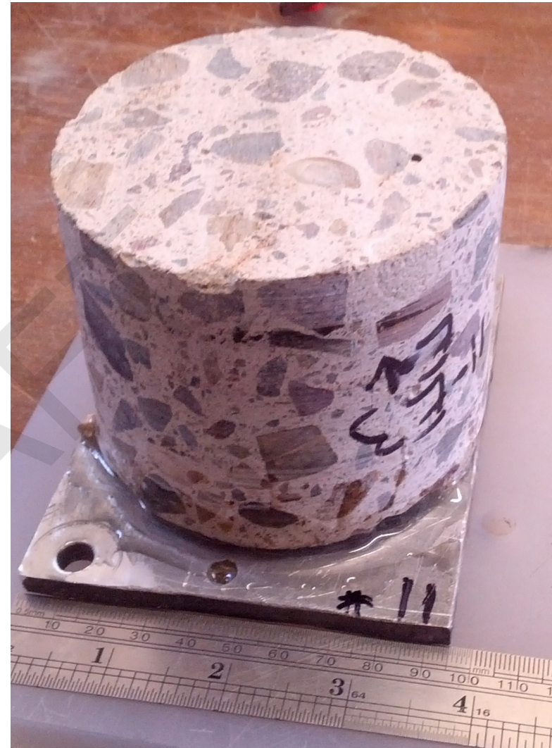
Core #11: Section for chloride analysis was cut at the observed reinforcement level. Reinforcement is located at about 2 1/4" below the exposure surface.
