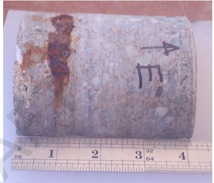
Core #14: Half core B (Pile Splash, Encasement) with embedded steel cable visible between sections 6 and 7. Half core B was not sectioned.
