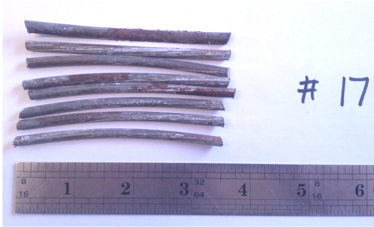
Recovered reinforcement elements (steel cable) of core #17
