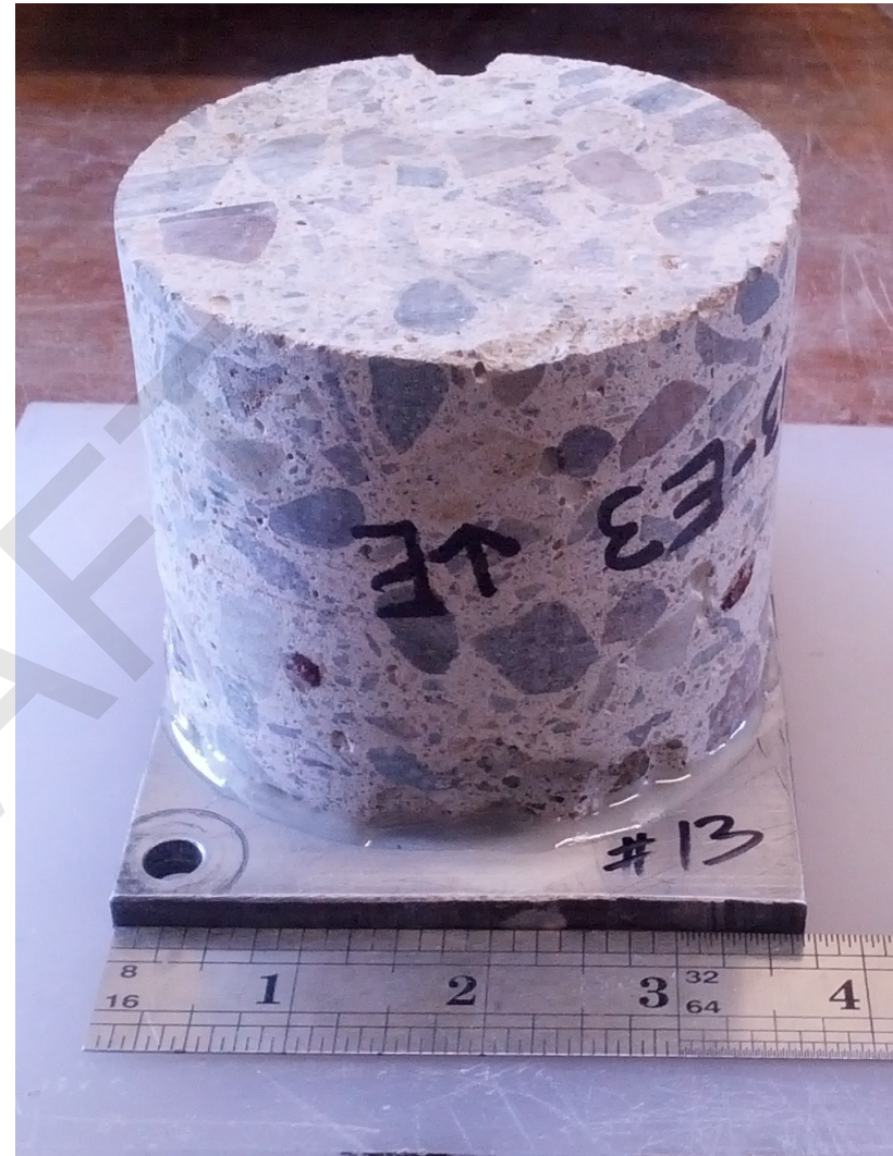
Core #13: Section for chloride analysis was cut at the observed reinforcement level. Reinforcement is located at about 1 7/8" below the exposure surface.
