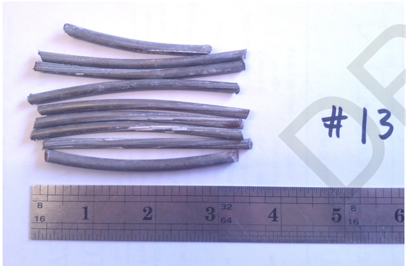
Recovered reinforcement elements (steel cable) of core #13
