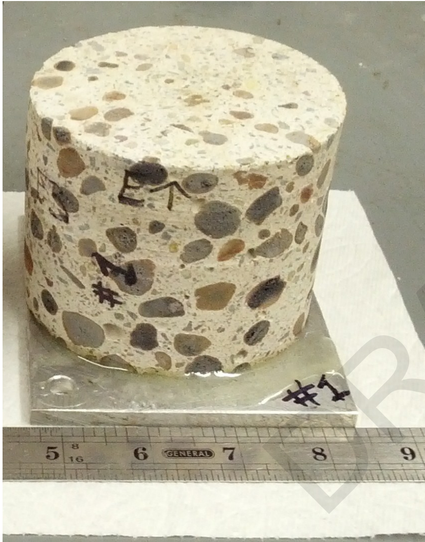
Core #1: Section for chloride analysis was cut at 1 3/4" from the exposure surface (bottom). No reinforcement was observed.
