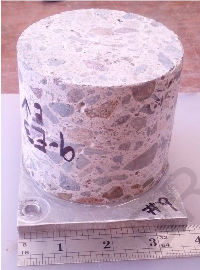
Core #9: As-received profile section mounted on Al base plate
