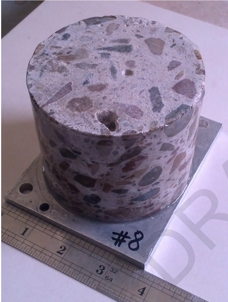
Exposure core #8: As-received profile section mounted on Al base plate
