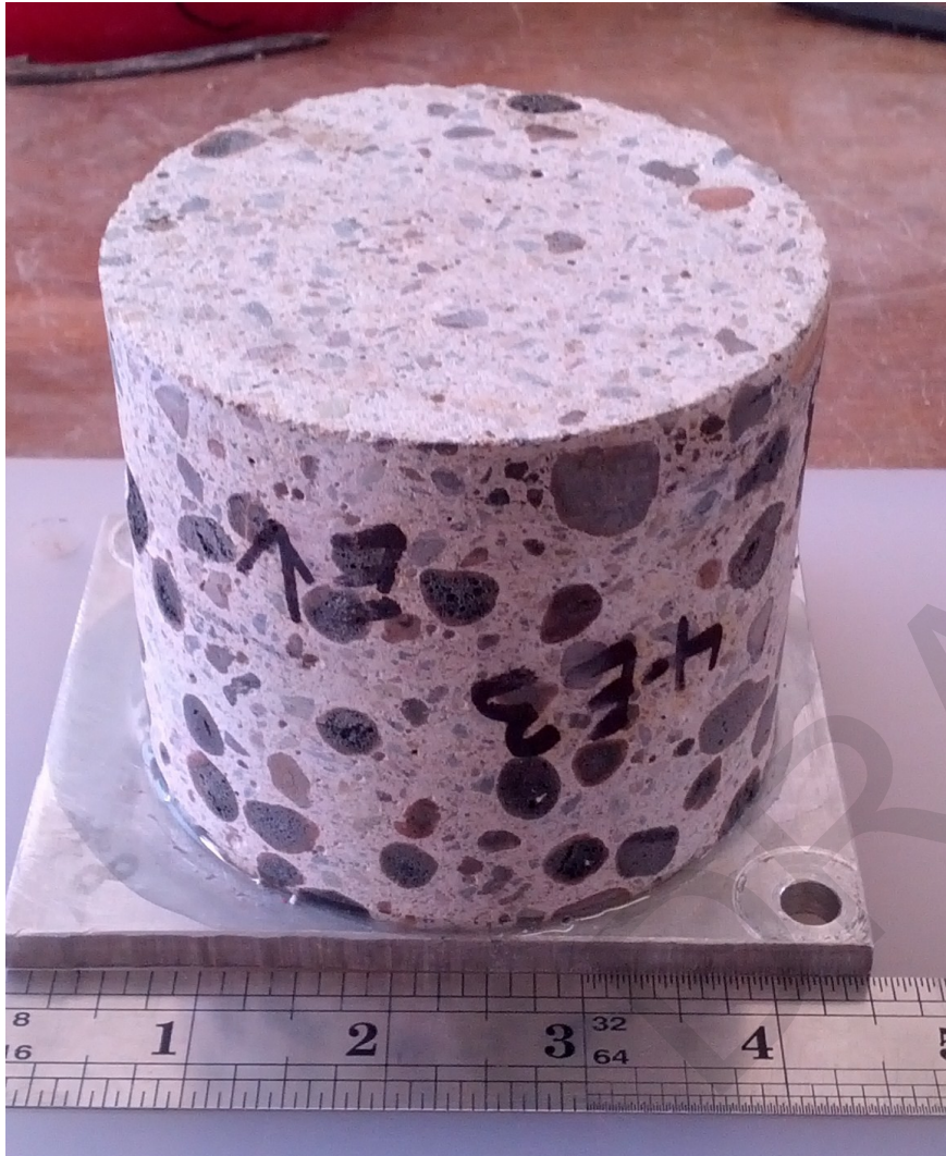
Core #4: As-received profile section mounted on Al base plate
