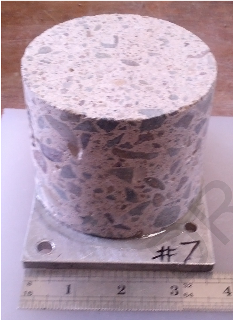
Core #7: As-received profile section mounted on Al base plate
