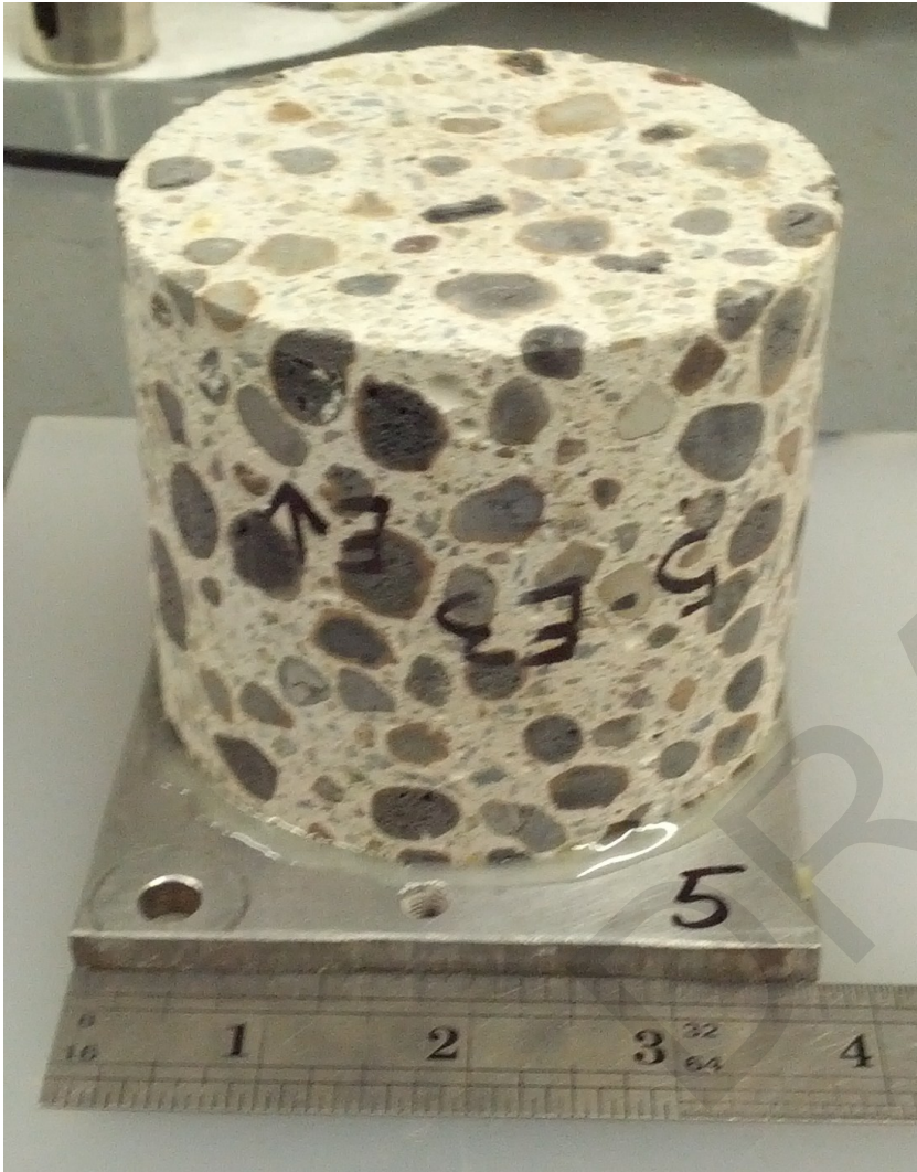
Core #5: As-received profile section mounted on Al base plate
