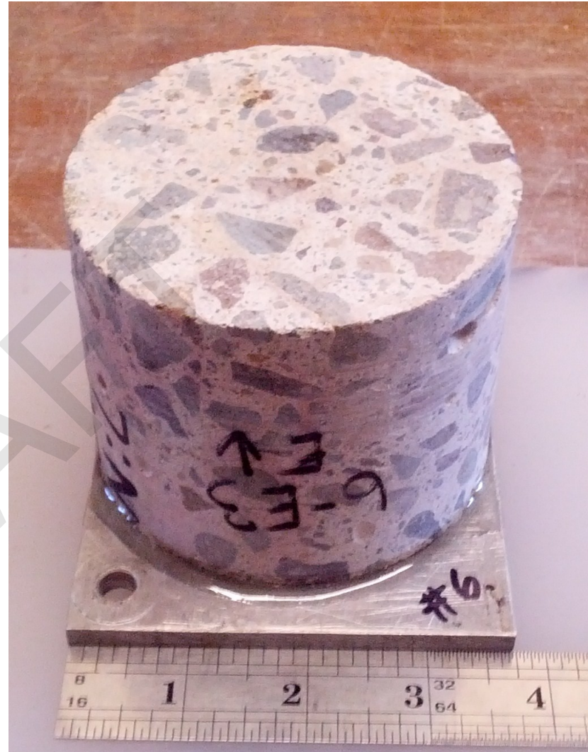
Core #6: As-received profile section mounted on Al base plate
