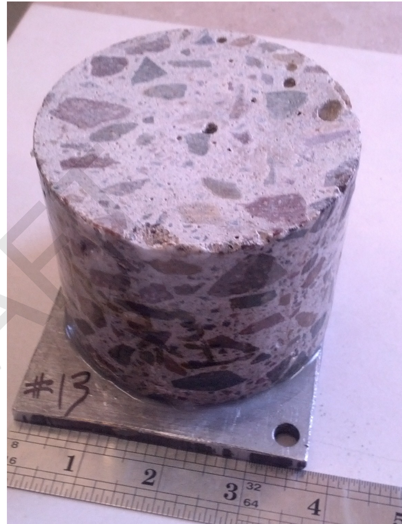
Exposure core #13: As-received profile section mounted on Al base plate
