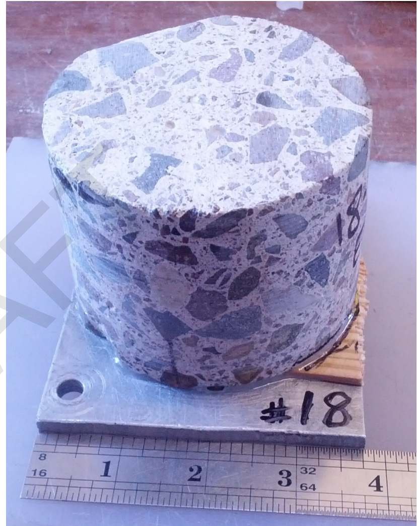
Core #18: Section for chloride analysis was cut at the observed reinforcement level. Reinforcement is located at about 2 \frac{1}{8} " below the exposure surface.
