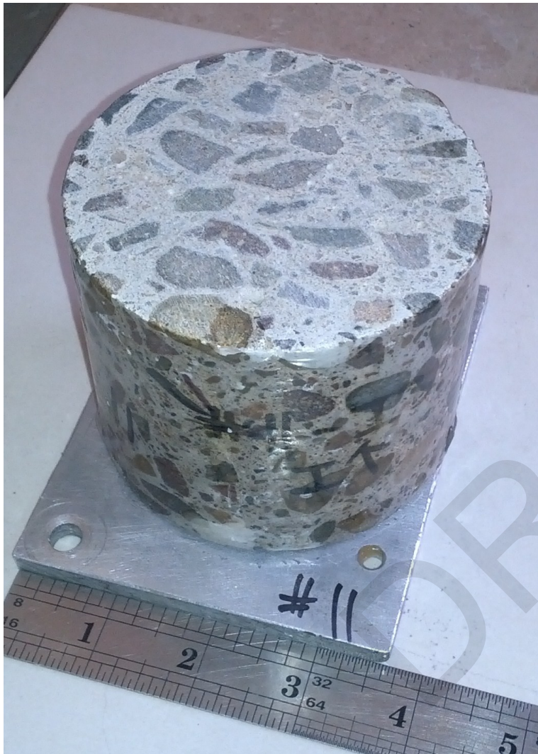
Exposure core #11: As-received profile section mounted on Al base plate
