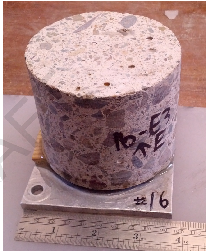
Core #16: Section for chloride analysis was cut at the observed reinforcement level. Reinforcement is located at about 2 3/8" below the exposure surface.
