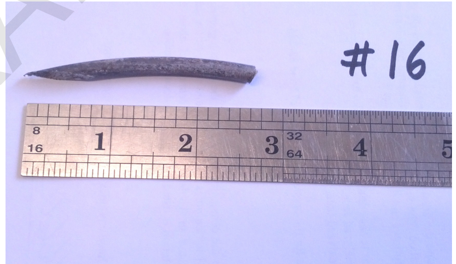
Recovered reinforcement elements (steel cable) of core #16
