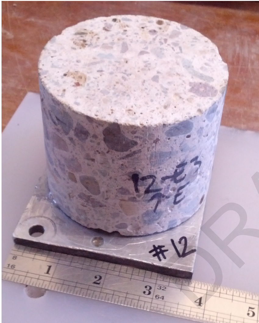
Core #12: Section for chloride analysis was cut at the observed reinforcement level. Reinforcement is located at about 2 1/4" below the exposure surface
