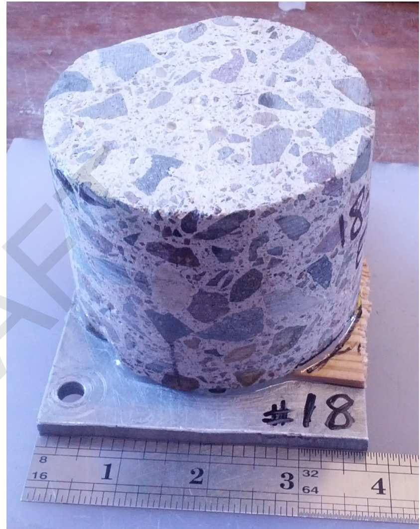
Core #18: As-received profile section mounted on Al base plate
