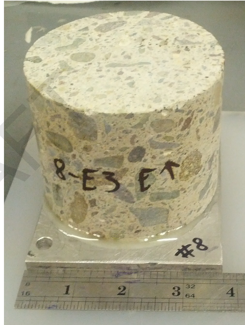
Core #8: As-received profile section mounted on Al base plate
