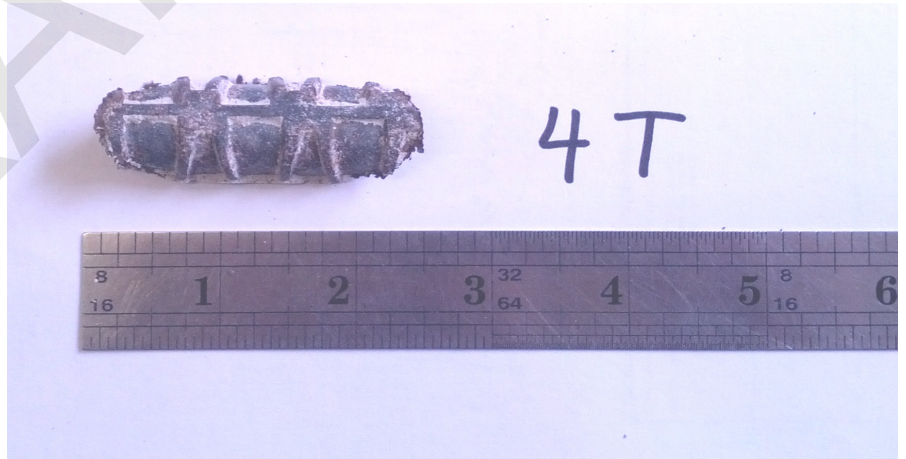
Recovered reinforcement element (steel rebar) of core #4T
