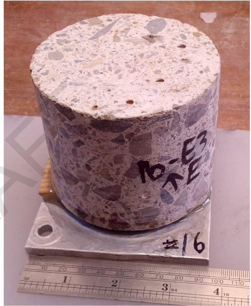
Core #16: As-received profile section mounted on Al base plate
