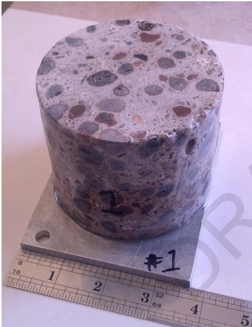
Exposure core #1: As-received profile section mounted on Al base plate
