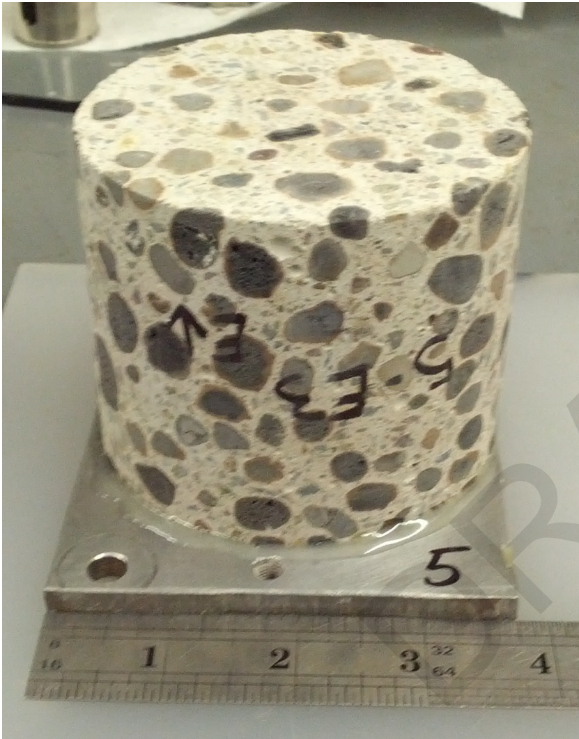
Core #5: Section for chloride analysis was cut at 1 3/4" from the exposure surface (bottom). No reinforcement was observed.
