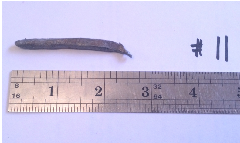
Recovered reinforcement elements (steel cable) of core #11
