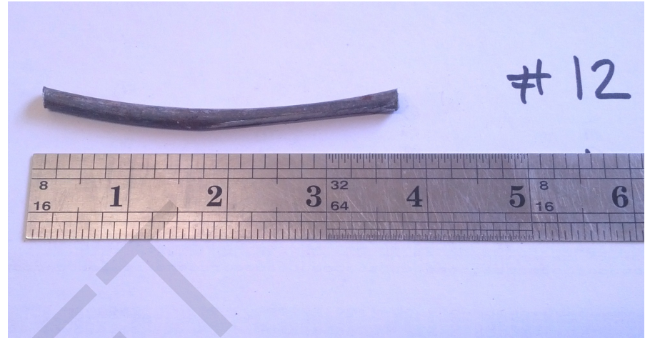
Recovered reinforcement elements (steel cable) of core #12
