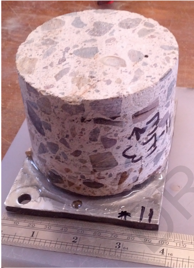
Core #11: As-received profile section mounted on Al base plate
