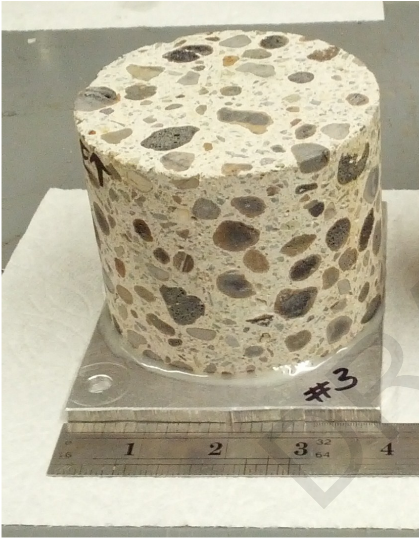
Core #3: As-received profile section mounted on Al base plate
