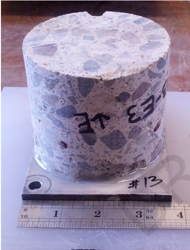
Core #13: As-received profile section mounted on Al base plate
