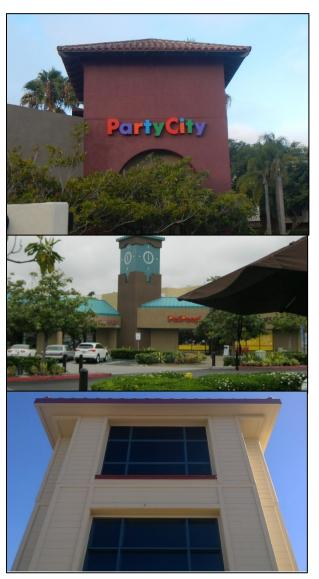
Figure 18: A cupola, a clock tower, and an added story, all concealing antennas. Note the replicated windows in the bottom picture.
