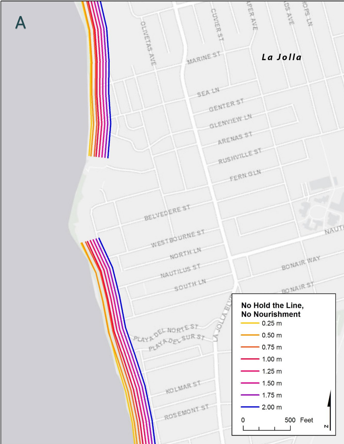
Figure 36. Detail of Figure 35. Coastal erosion given no protection at various levels of SLR at La Jolla.
