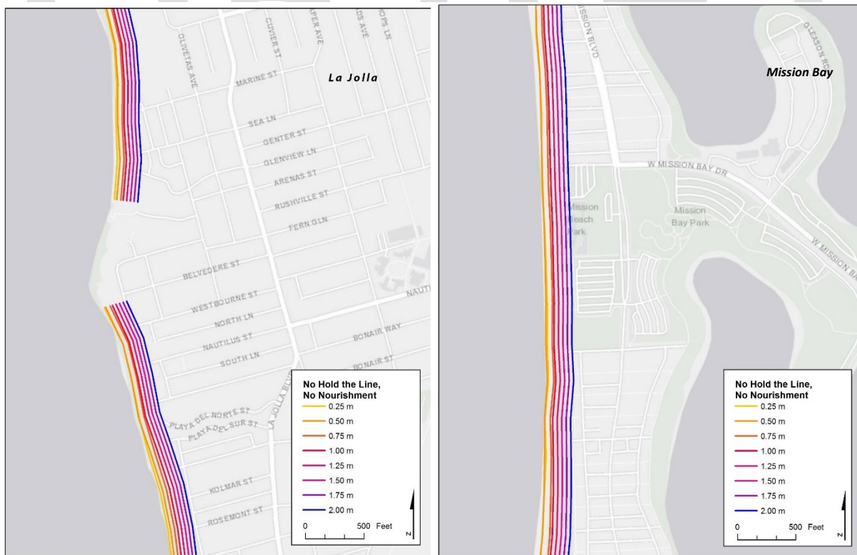
Figure 5. Coastal erosion scenarios given no protection and varying levels of SLR at La Jolla (left) and Mission Bay (right.) Larger maps are available in the Appendix. Source: ICF, based on SanGIS and CoSMoS data
