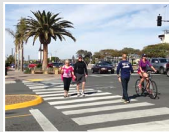
High visibility crosswalk clearly indicates pedestrian activity
