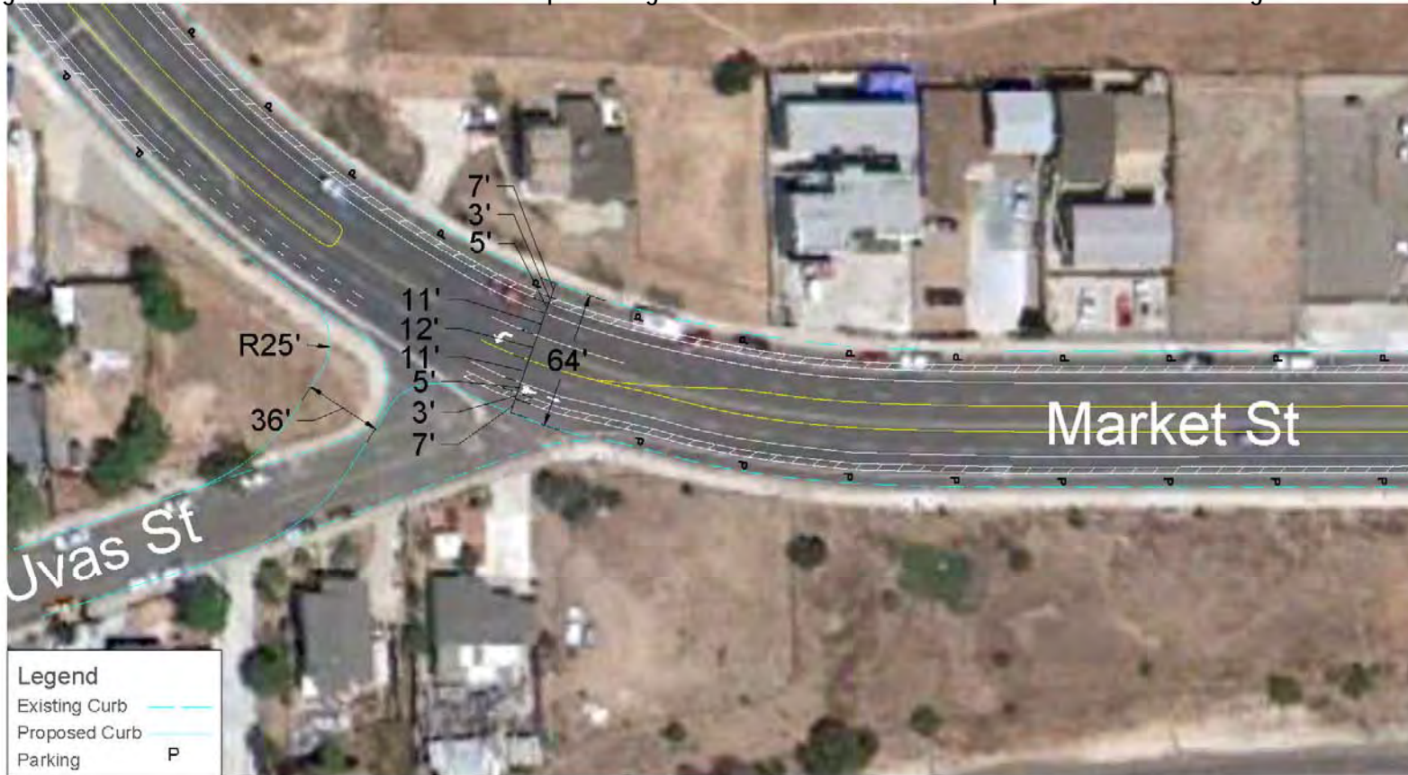
Figure 3-8a Market Street at Uvas: Initial Draft Concept Drawing of Interim Road Diet with Conceptual Intersection Redesign 9
