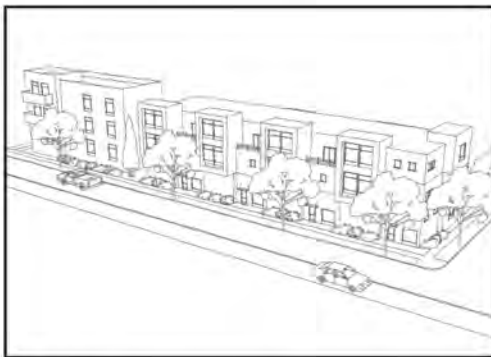
Articulation: The character of a building can be better articulated by coordinating window locations and sizes with the massing.
