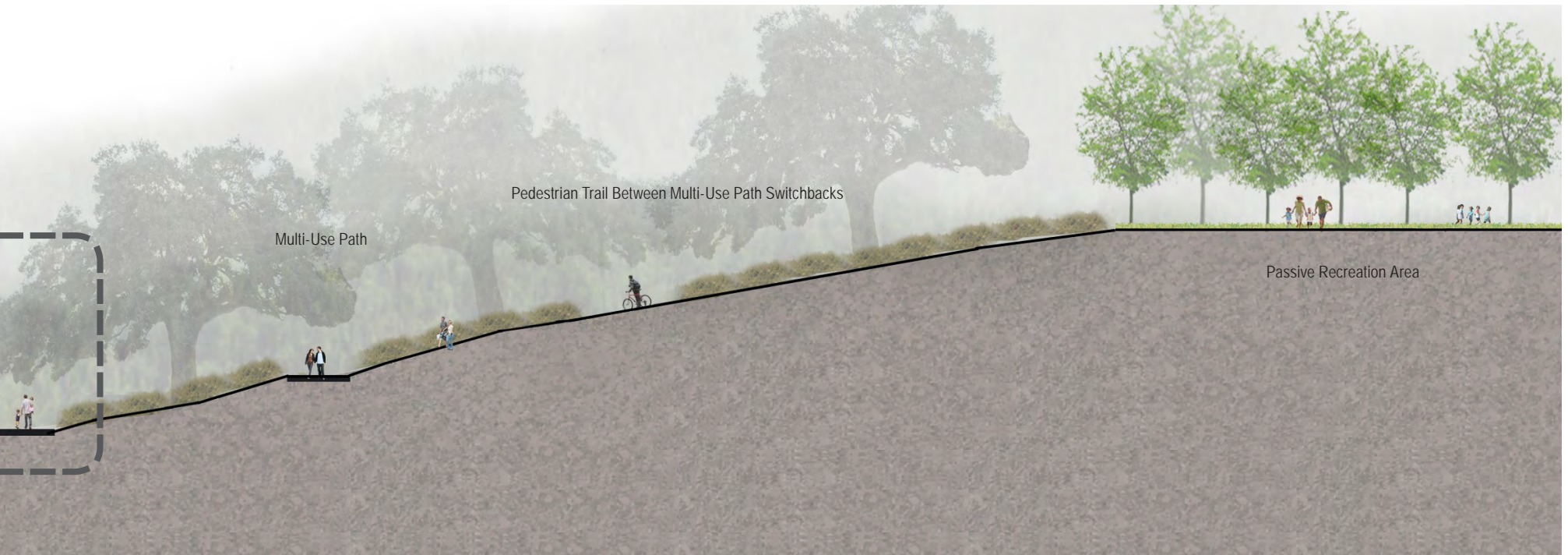
Example of pedestrian trail stairs connecting between multi-use trail switchbacks made of recycled concrete
