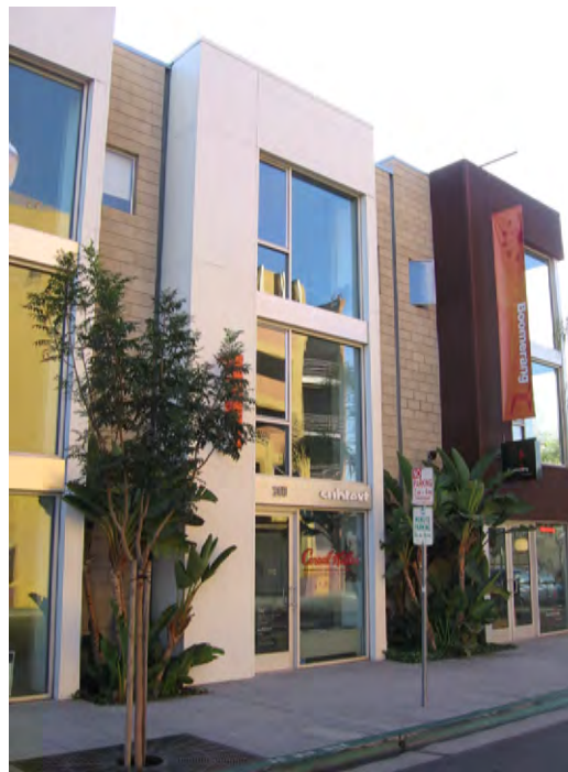
Break down building massing with a change in materials and forms that define a rhythm of bays and sections of a building.
