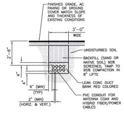
NOTE: PROVIDE PROPER BENDING RADIUS FOR CONDUITS AS REQUIRED BY THE COAXIAL CABLE MFR.
