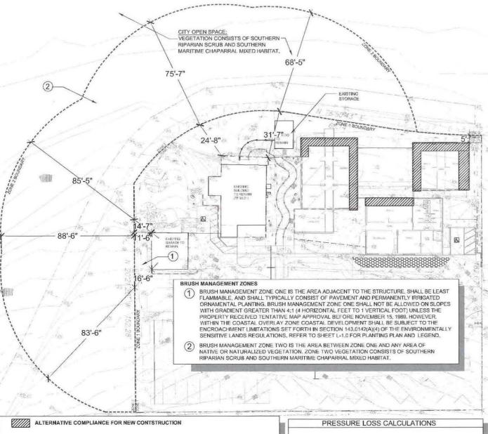
BRUSH MANAGEMENT SHALL NOT BE ALLOWED ON CITY OPEN SPACE FOR NEW CONSTRUCTION. OPENING PROTECTION ALONG FACES SHOWN SHALL BE UPGRADED TO DUAL-GLAZED. DUAL TEMPERED PANES OR GLASS BLOCKS IN ADDITION TO CBC 7A REQUIREMENTS. SEE ARCHITECTURAL PLANS SHEET A1.1 DEPUTY FIRE MARSHAL SIGNATURE. DATE
