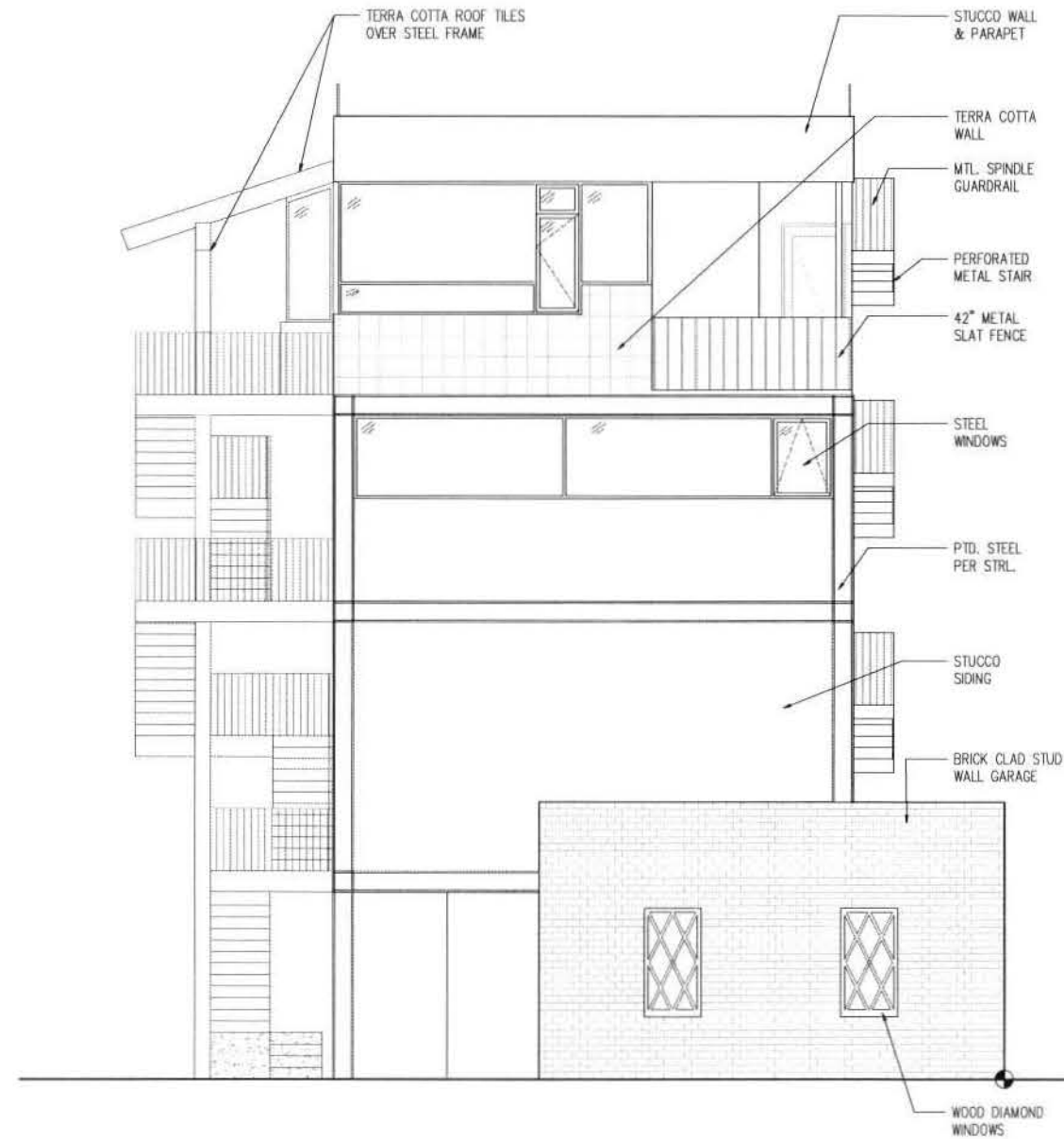
② BLDG M - EAST ELEVATION @ STREET SCALE: 1/4"=1'-0"
