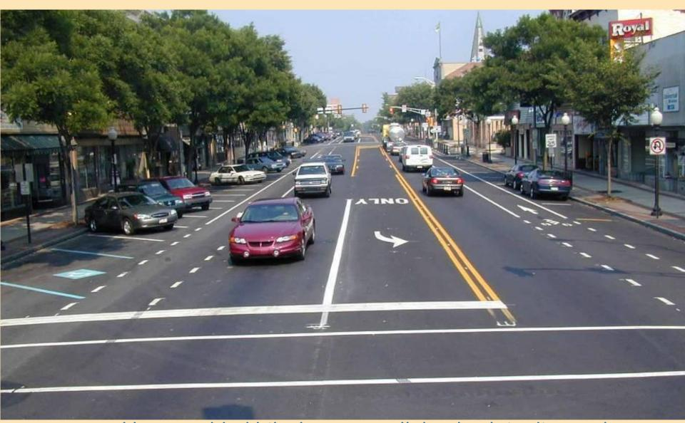
Fewer travel lanes; added bike lanes; parallel to back-in diagonal parking on one side; new pavement
