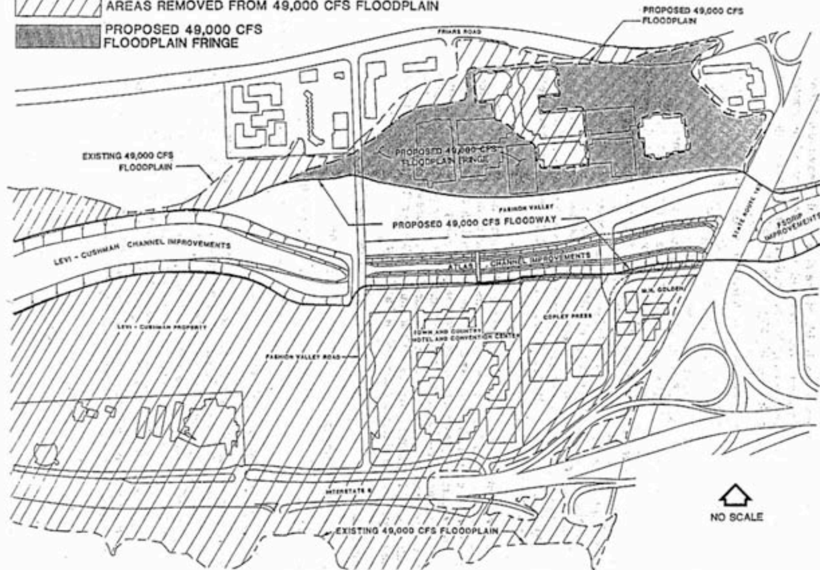
Existing and Proposed Floodplain and Floodway with FSDRIP, Atlas and Levi-Cushman Improvements
