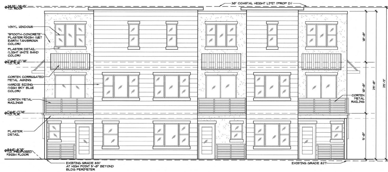
1 ENTRY ELEVATION - BLDG B SCALE: 1/4" = 1'-0"
