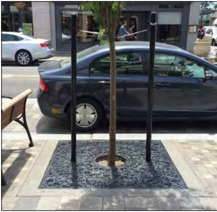
Small to Large Tree with Tree Grate
