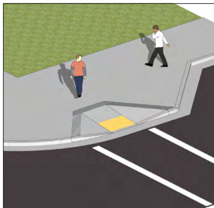
Pedestrian Ramp and Bulbout (Midblock or Intersection)
