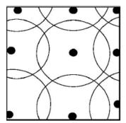
FIGURE 2-2 SPRAY DIAMETER IN TURF AREA
